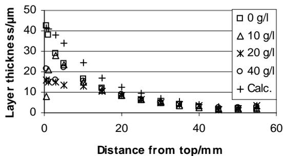
**Figure 2. Zn Layer Thickness as a Function of the Distance from Top of RCHC**
