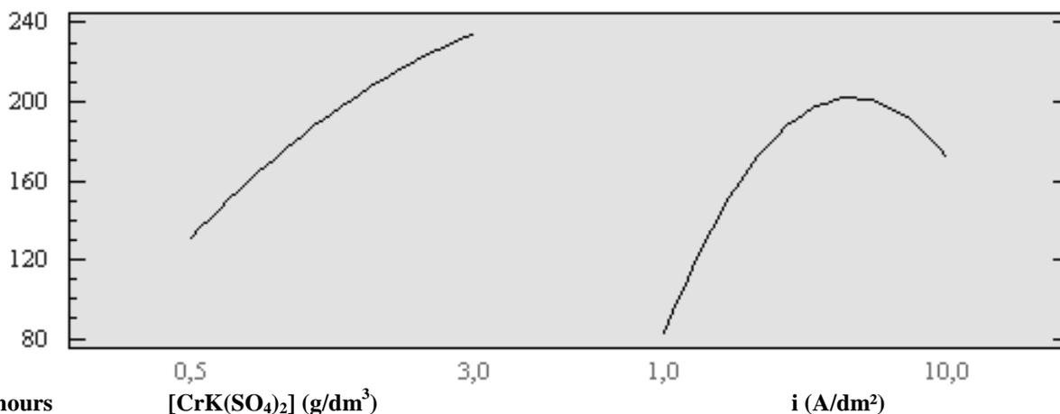
**Figure 6.** Main effects plot for first appearance of red rust in NSS.
