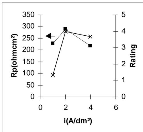
**Figure 5. Main Effects Plots for Corrosion Tests.  $R_p$  measured by EIS. Rating in NSS after 168 hours exposure.**
