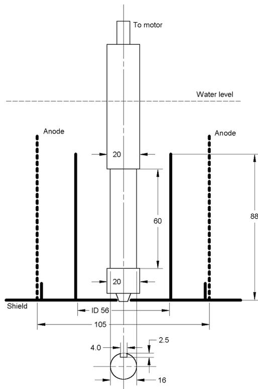
**Figure 1. The Rotating Cylinder Hull Cell**
