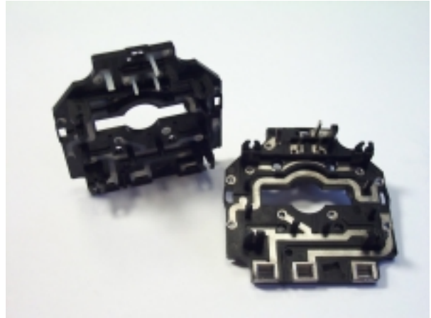
Figure 5 - MID-Component of a Control Gear (Electric Motor; 250 V), PA (by Courtesy of J. Stehle + Söhne AG)
