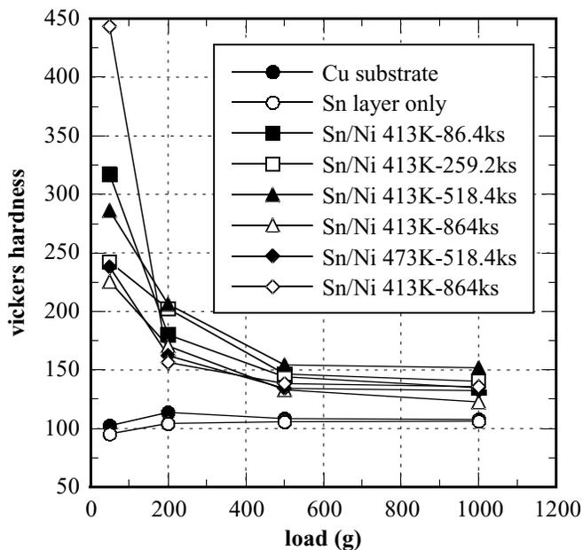
Fig. 8 Vickers hardness of specimens with Cu substrates.
