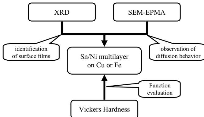
Fig. 3 Experimental procedure.
