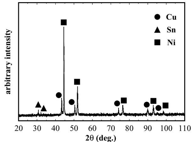
Fig. 5 XRD result for Ni/Sn multilayered copper before heating (Sn: 1 A/dm<sup>2</sup>, Ni: 5 A/dm<sup>2</sup>).
