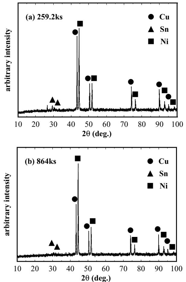
Fig. 7 XRD result for Ni/Sn multilayer on copper heated at 473°K.
