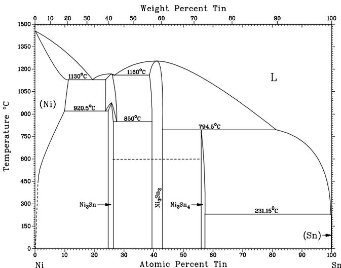
Fig. 1 Phase diagram for Ni-Sn.
