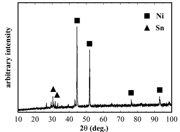
Fig. 10 XRD result for Sn/Ni/Cu heated in 864ks.
