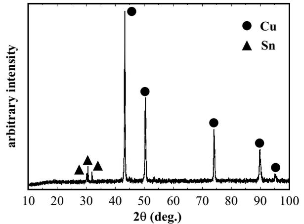
Fig. 4 XRD result for Sn plated copper (at 1 A/dm<sup>2</sup>).
