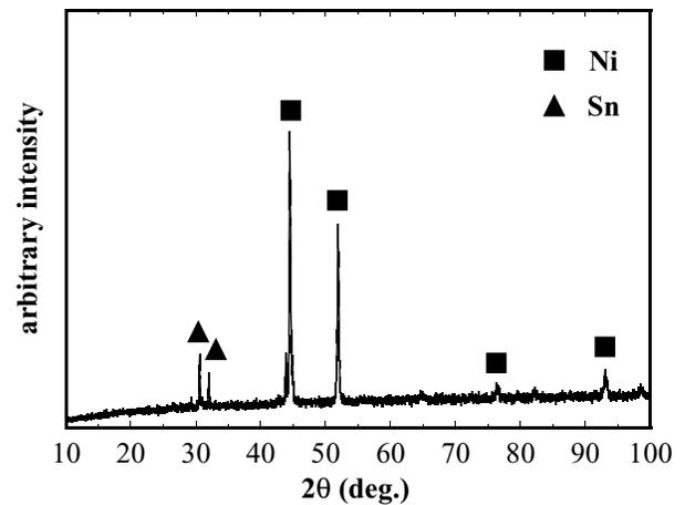
Fig. 9 XRD result for Sn/Ni/Cu before heating.
