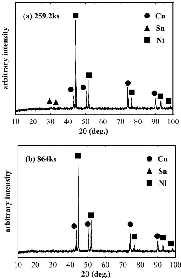
Fig. 6 XRD result for Ni/Sn multilayer on copper heated at 413°K.
