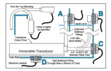
Electrical connections from the transducers to the ultrasonic generators are made using solid or flexible stainless steel tubing. An alternative scheme involves penetrating the tank wall directly behind each transducer with a gasketed bulkhead fitting. This method is less convenient as it requires draining the tank for transducer repair or replacement if needed.
