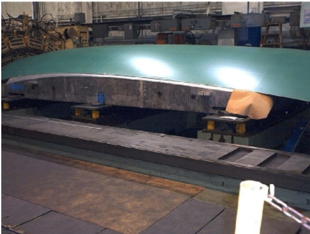
Photo 3 Complex contour stretch formed masked part 113" X 300" X 0.170" Photo 4
