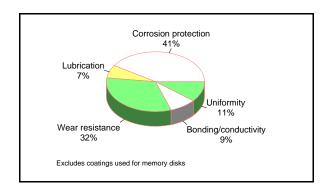
Figure 6 shows the results of a survey conducted in 1993 of job shop and captive facilities in the United States to find the types of parts plated and the industries that use them. By far the largest users of electroless nickel coatings are the memory disk manufacturers. These facilities apply more than one fifth of all of the coatings in the United States. Little if any of this type of plating is done in job shops.
