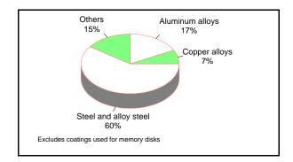
In job shops, most of the work is on ferrous substrates. Approximately 60 percent of the parts that are plated are made from plain steel, iron and alloy steels. This equals a reduction of one quarter from that reported in 1979<sup>18</sup>.
