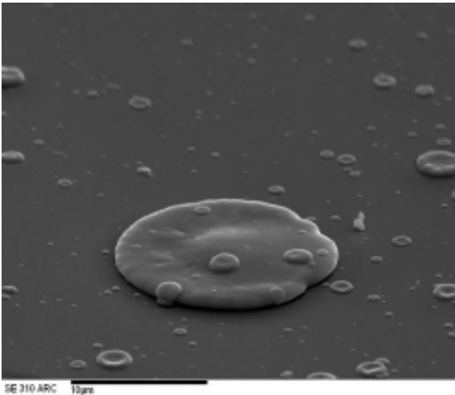
**Figure 10b:** Arc Deposited Stainless Steel
