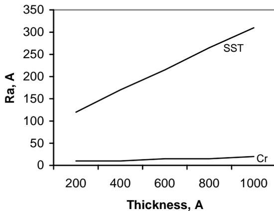
**Figure 13:** Thickness vs Roughness (Ra) - Arc
