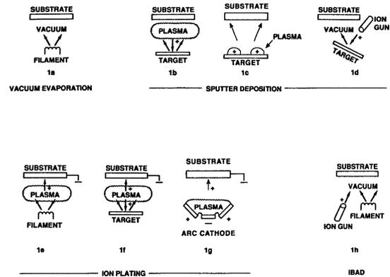
**Figure 1.** PVD processing techniques: (1a) vacuum evaporation, (1b and 1c) sputter deposition in a plasma environment, (1d) sputter deposition in a vacuum, (1e) ion plating in a plasma environment with a thermal evaporation source, (1f) ion plating with a sputtering source, (1g) ion plating with an arc vaporization source and, (1h) ion beam assisted deposition with a thermal evaporation source and ion bombardment from an ion gun.
