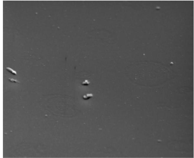
**Figure 9a:** Sputter Deposited Aluminum
