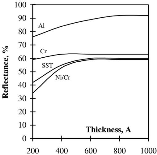
**Figure 12.** Thickness vs Reflectance - Sputtering
