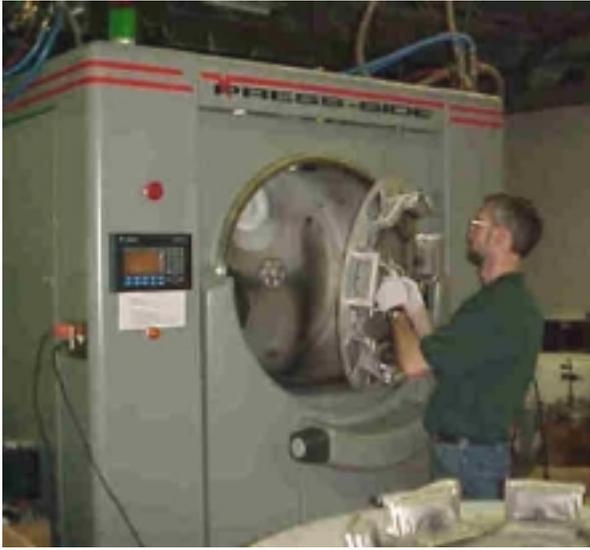
**Figure 5.** Sputtering and Arc Coating System
