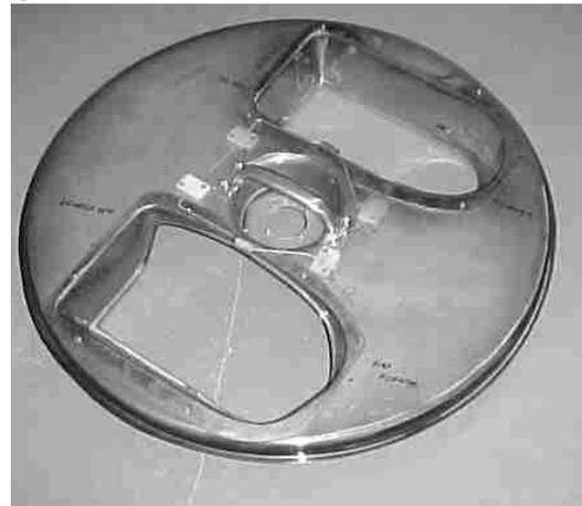
**Figure 8.** Vacuum Formed PETG Disc
