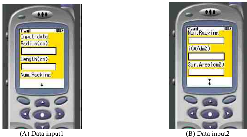
Fig.2 Calculation of surface area and total current
