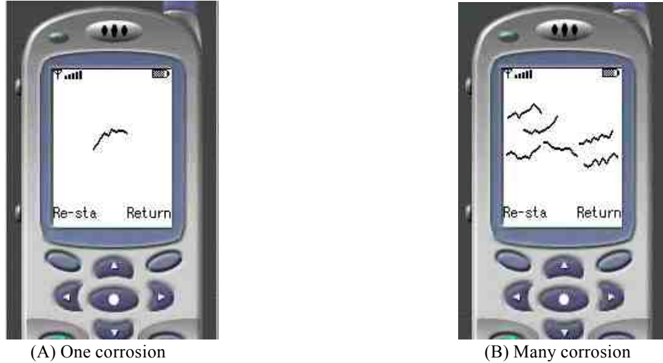
Fig.18 Patterns of filiform corrosion by Monte-Carlo simulation
