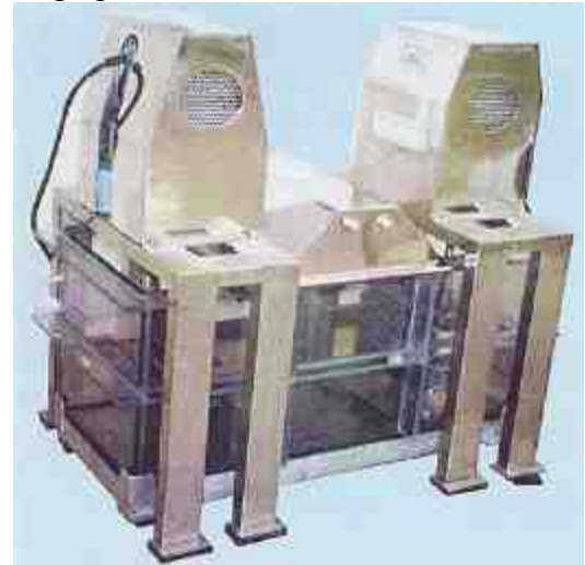
Photo.5 Sterilization equipment by photocatalyst function of titanium oxide film
