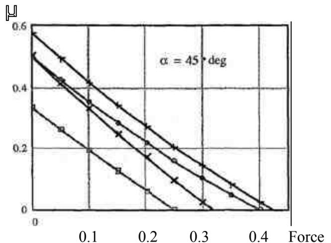
Figure 4. Centering dynamic force vs. coefficient of friction.
