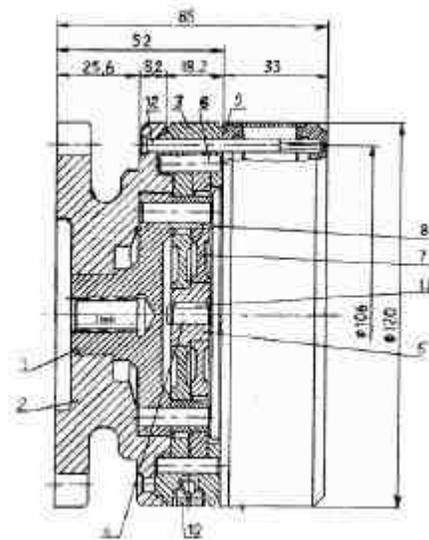
Figure 2. Brake disk in detailed view.
