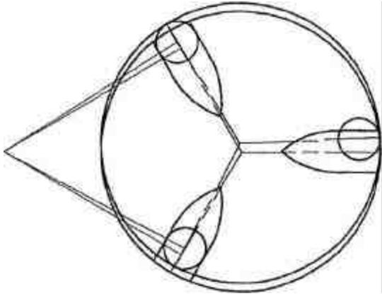
Figure 5. The limiting case for centering occurs when three steel break pads contact the alumina surface of the disk.
