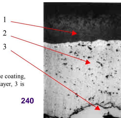
Figure 1. Microstructure of the composite coating, where 1 is alumina layer, 2 is aluminum layer, 3 is rough steel base.
