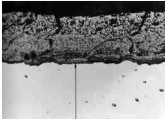
Fig. 3. Initial cracks formed in the alumina layer.
