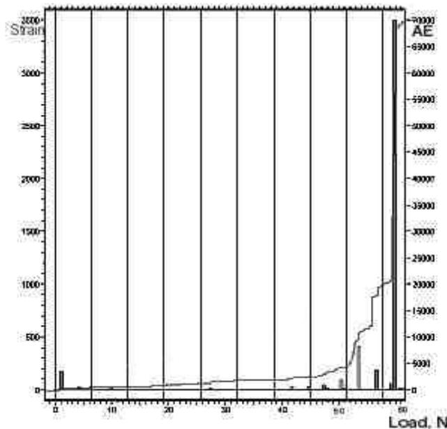
FIG. 2. Acoustic emission and strain vs. applied load.
