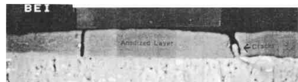
Figure 1. SEM micrograph of alumina layer with cracks.
