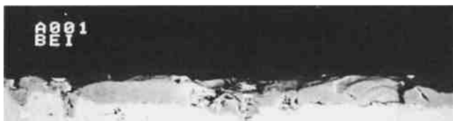
Fig 5. SEM micrograph of alumina layer showing the distribution of precipitates and cracks across the layer (perpendicular to the surface).
