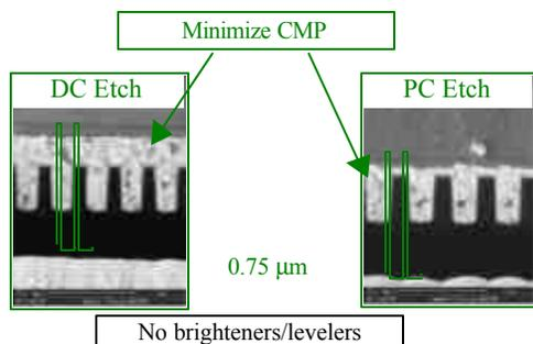
Figure 10 – Minimization of overplate/CMP, by control of etching step.
