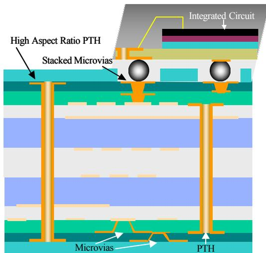
Figure 1 - Schematic of Advanced Electronic Package.
