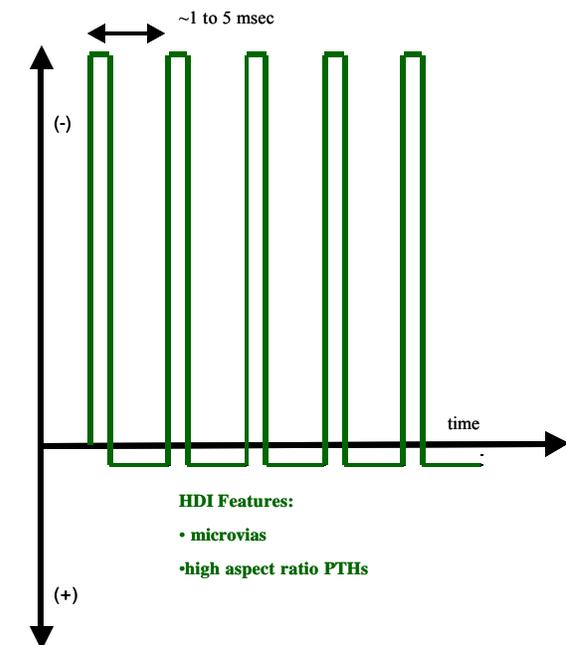
Figure 3 - Generalized Waveform for High Aspect Ratio PTHs and Microvias.
