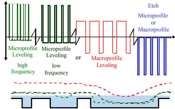
Figure 7 – Variety of electrically mediated processes which can be applied to metallization of VLSI features.
