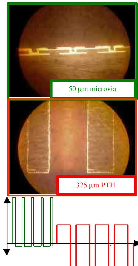
Figure 5 – Metallization of 50  $\mu\text{m}$  microvia and 325  $\mu\text{m}$  PTH, in one process step using waveform sequencing.
