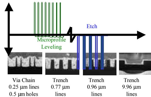
Figure 8 – Metallization of various IC features, using electrical mediation and waveform sequencing.
