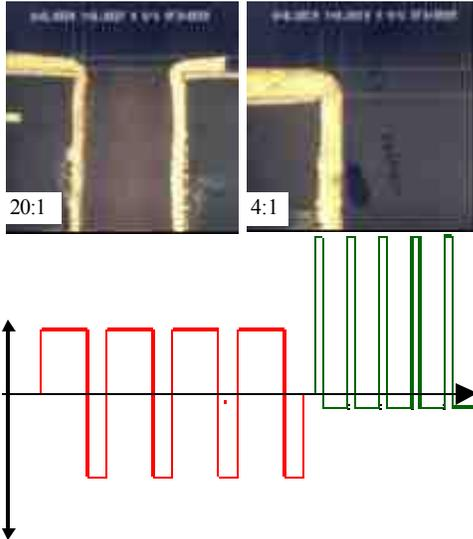
Figure 6 – Metallization of 20:1 and 4:1 PTHs, using waveform sequencing.
