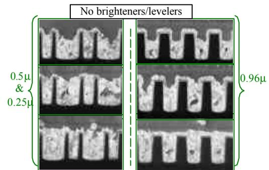
Figure 9 – Metallization of IC features, using electrical mediation, with minimal overplate/CMP.
