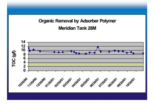
As can be seen, the TOC was held between 8 and 12 g/l. Throughout this time the deposit ductility specification of 11% or greater was never violated. No F006 waste from batch carbon treatment was created because no batch carbon treatments were performed. The solutions from the regeneration of the adsorber polymer are easily treated in Meridian's waste treatment system for nickel plating.
