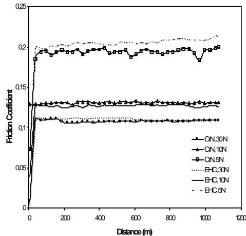
Figure 1. Friction coefficients of CrN and EHC vs. distance (m) at room temperature for all loads
