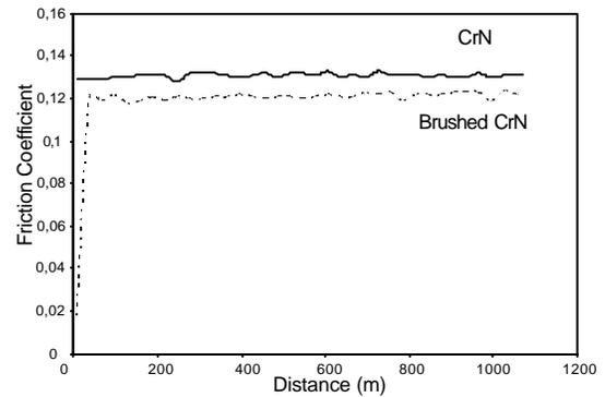
Figure 9. Friction coefficients of CrN and brushed CrN coatings vs. distance
