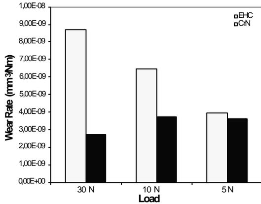
Figure 5. Wear rates of steel balls sliding against EHC and CrN coatings, for all loads at 60°C.
