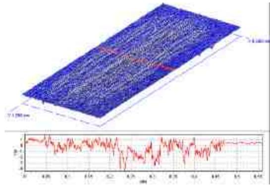
Figure 6. The 3D and 2D wear scar profiles on EHC coated disc, at 30N load and 60°C
