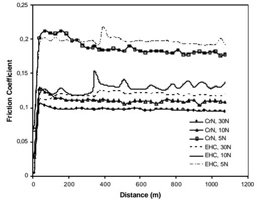
Figure 2. Friction coefficients of CrN and EHC vs. distance (m), at room temperature for all loads
