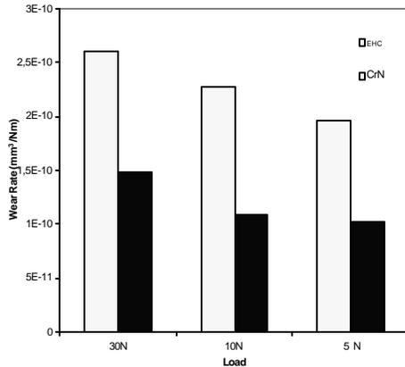
Fig. 3. Wear rates of steel balls sliding against EHC and CrN coatings, for all loads at room temperature
