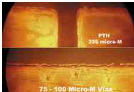
Fig. 15 Two sided PCB with PTH and blind via features
