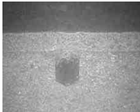
Fig. 14 Incorrect waveform parameters or the incorrect sequence of waveforms can block access to smaller features
