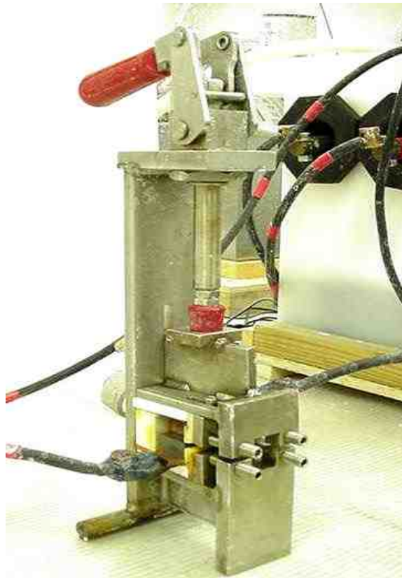
Figure 2. Schematic of Experimental Setup for Electrically Mediated Finishing and Electrolyte Flow Path on Workpiece Surface using Wedge Shape Tool.
