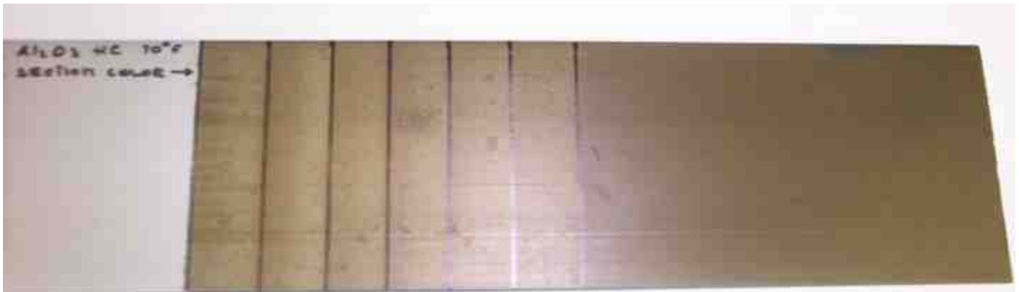
6061-T6511 aluminum alloy with 0.2-0.3 mils of hard coating by DC+AC process (70°F) and electrolytic coloring
