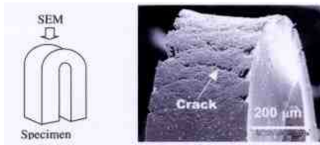
Fig. 1 Preparation of specimens for observation of the fractured section of the deposits.
