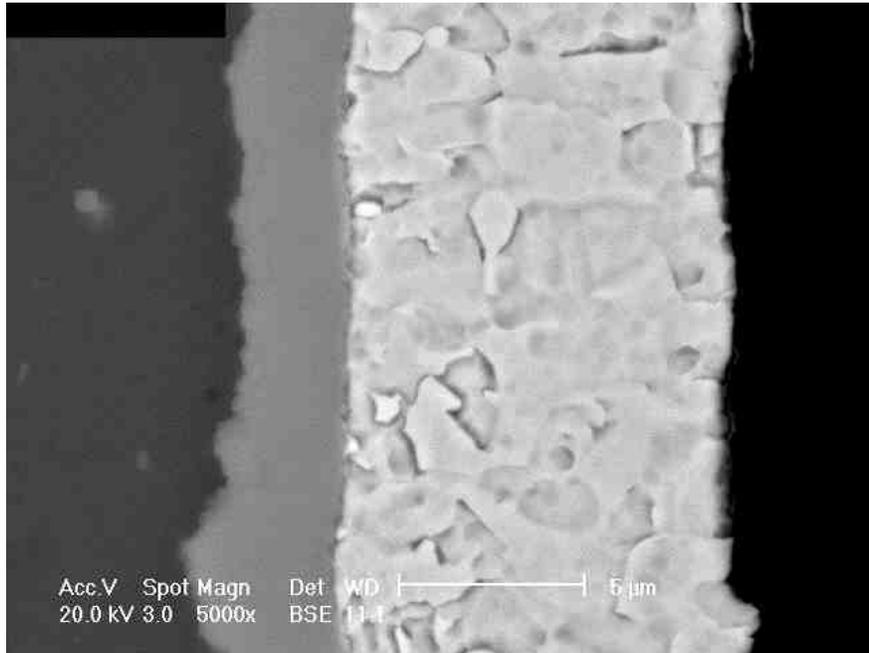
Fig. 4: Cross-section of a galvanic nickel layer (bright, on the right) on aluminium (dark, on the left) after heat treatment. The diffusion layer between them is clearly visible (grey)
