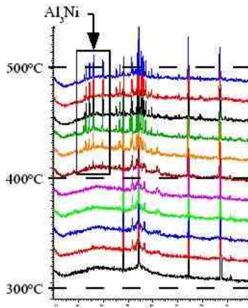
Fig. 3: In-situ high-temperature XRD measurement of the Ni-Al boundary
