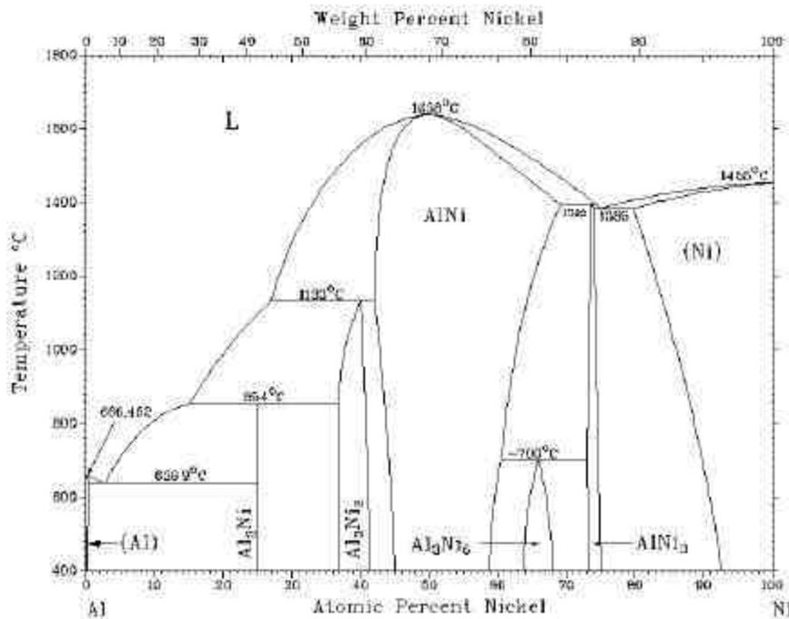
Fig. 1: Binary Alloy Diagram Nickel-Aluminium.
