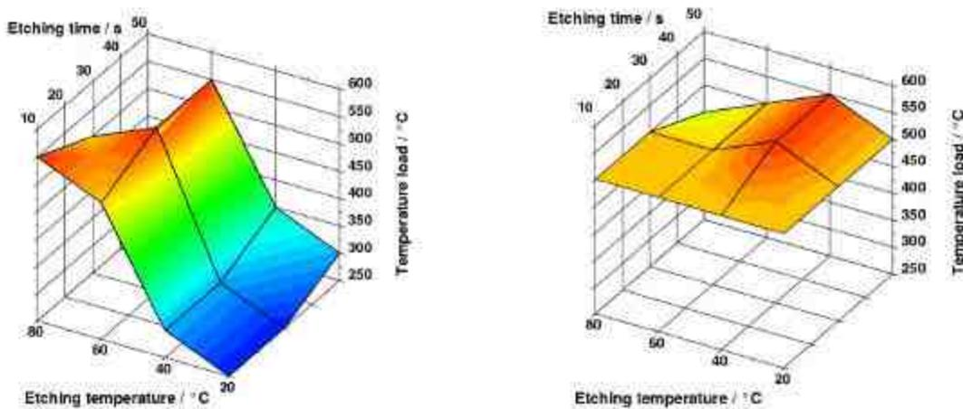
Fig. 2: Optimum Fe-pickling conditions for galvanic nickel (left) and electroless Nickel (right) on aluminium based on temper test results.
