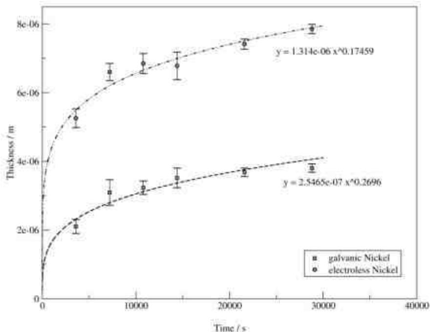
Fig. 5: Growth process of  $Al_3Ni$ -layers during temper experiments at 500 °C
