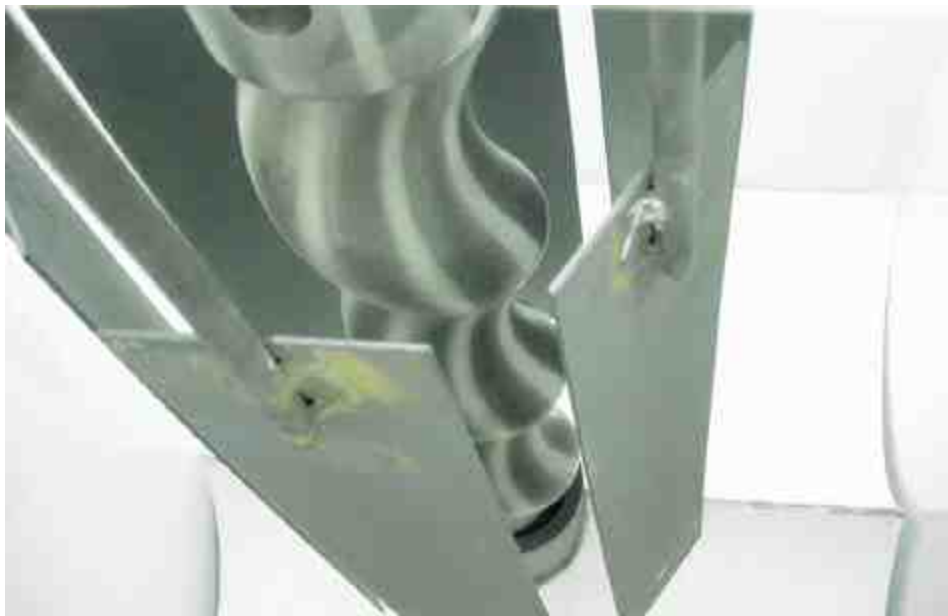
Figure 6: Plating set-up for pump augers
