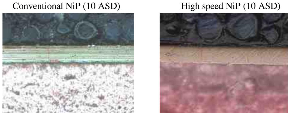
*Fig. 14 Cross section of different NiP layers*
