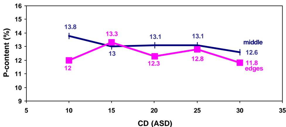
Fig.8 P-content depending on CD (Substrate plated in a reel to reel line)
