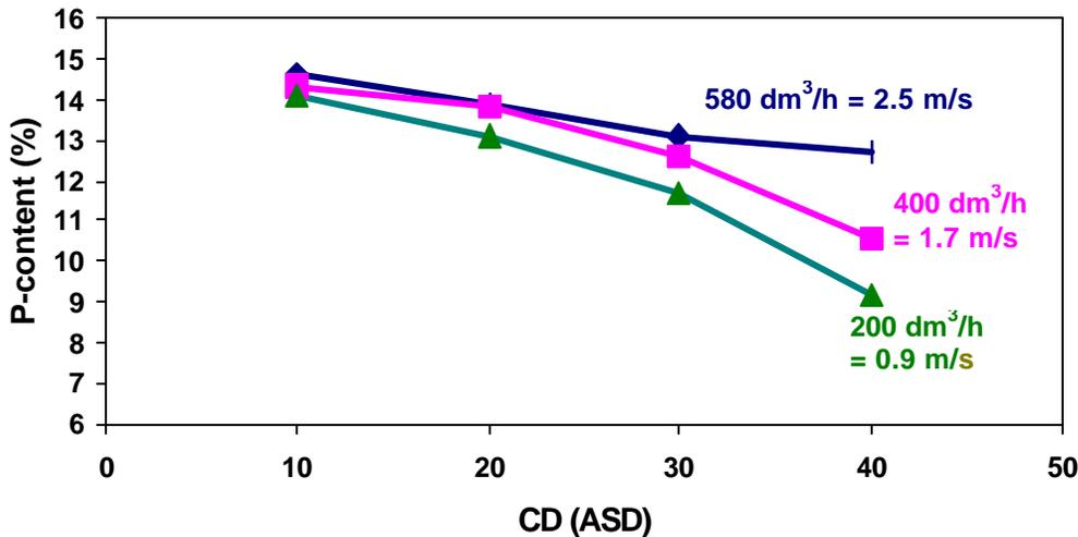
Fig.4 P-content depending on flow rate and current density (CD)
