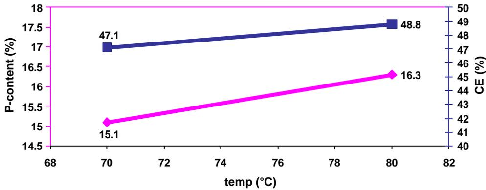
Fig.6 P-content and current efficiency depending on temperature
