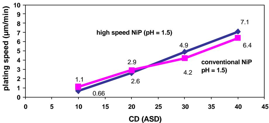
Fig.2 Plating speed depending on current density (CD)
