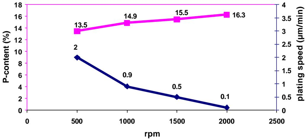
Fig.5 P-content and plating speed depending on speed of rotation
