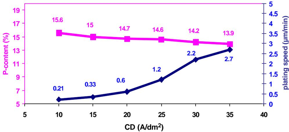
Fig.3 P-content and plating speed depending on current density (CD)
