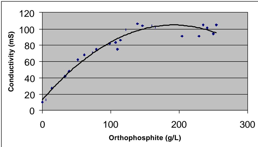
Fig. 3. Conductivity of waste salt solution (Tank C2) with increasing sodium orthophosphite concentration.
