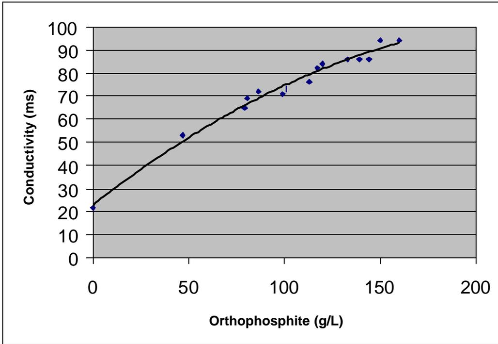
Fig. 2. Conductivity of electroless nickel process with increasing sodium orthophosphite concentration.
