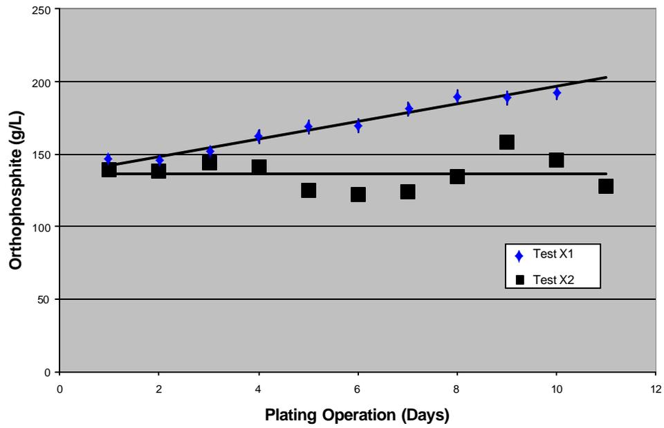
Fig.3. Sodium Orthophosphate concentration for tests during electrolysis maintenance tests X1 and X2 over time.
