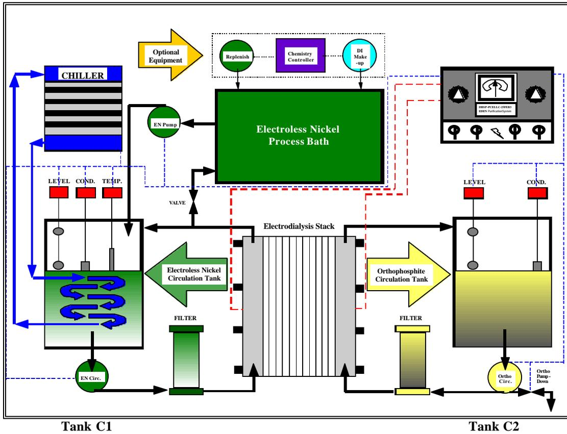
*Fig. 1. Schematic of the Continuous Low Temperature ED system.*
