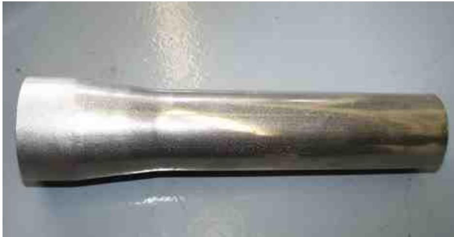
Figure 4. Plain carbon steel pipe having a 0.010 in. OD coating of nanocrystalline Ni (15nm grain size) which has been cold-swaged (rotary) from a 2.5 in. to 2.0 in. diameter in a single step.
