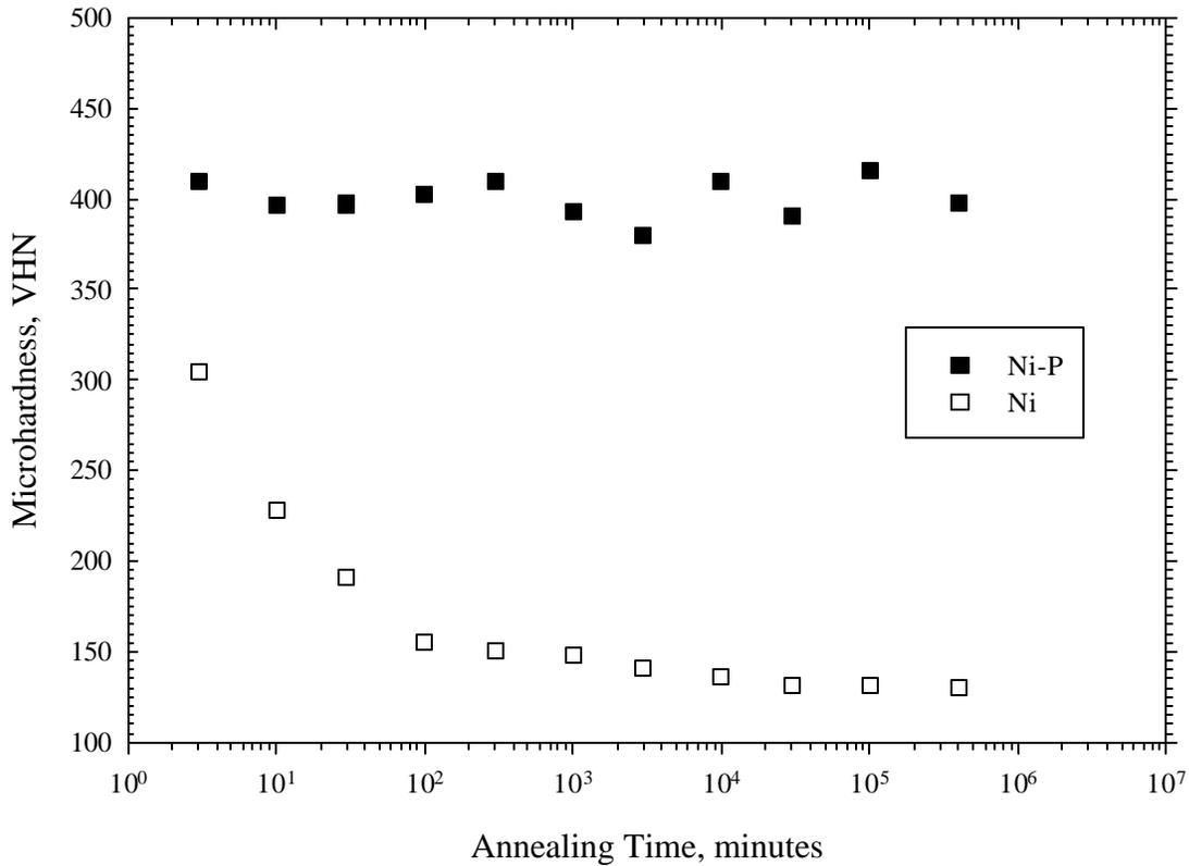
Fig. 2 – Vickers hardness as a function of annealing time at 343°C (650°F) for nanocrystalline (1) Ni and (2) Ni-1500P<sup>5</sup>.
