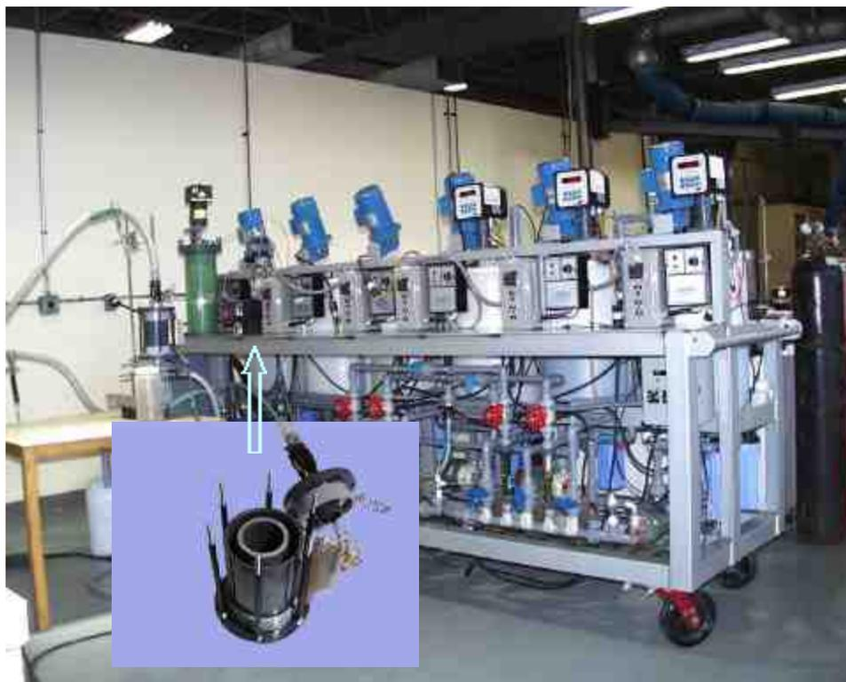
*Fig.5 – Photograph of the portable plating rig along with an early plating cell prototype (inset).*
