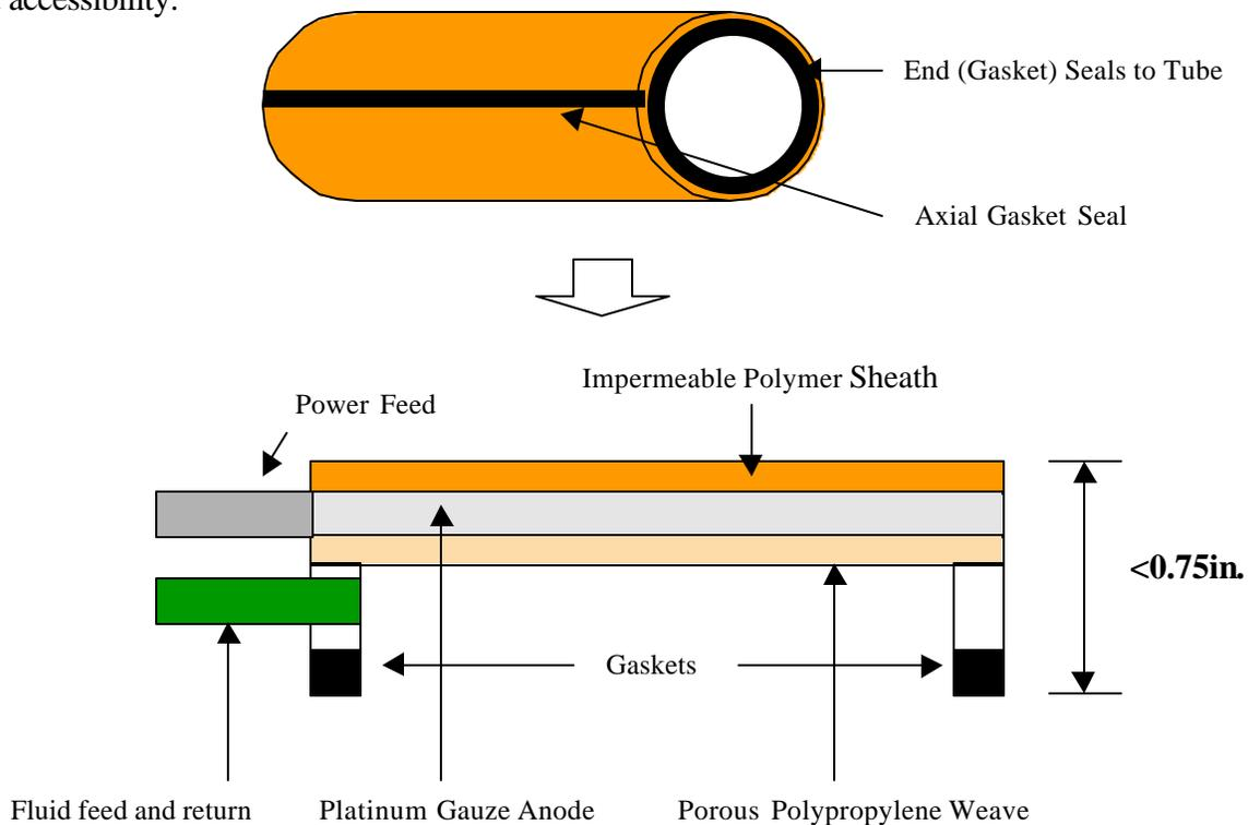
Fig. 4 – OD pipe plating cell – flexible jacket concept
