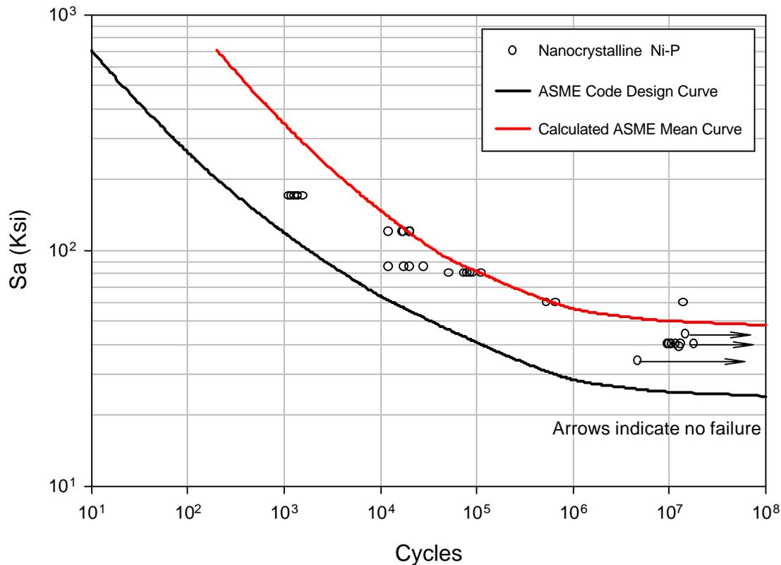
Fig. 3 – Comparison of nanocrystalline Ni-P fatigue test data to the ASME fatigue design<sup>9</sup> and mean curve for austenitic stainless steels and nickel-based alloys (Tests were performed in fully reversed bending ( $R=-1$ )). Arrows denote no sample failure.
