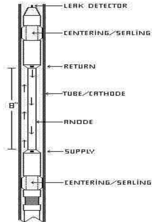
Fig. 1 – Electro-sleeve probe for in-situ structural repair of degraded steam generator tubing.
