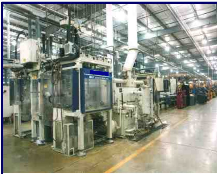
Figure 11 Electrolytic Machining Equipment Processing Airbag Housings
