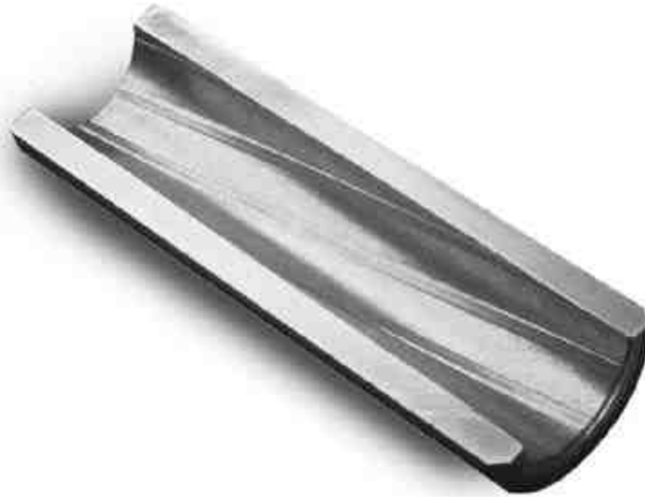
Figure 16 b Electrolytically Formed Rifling
