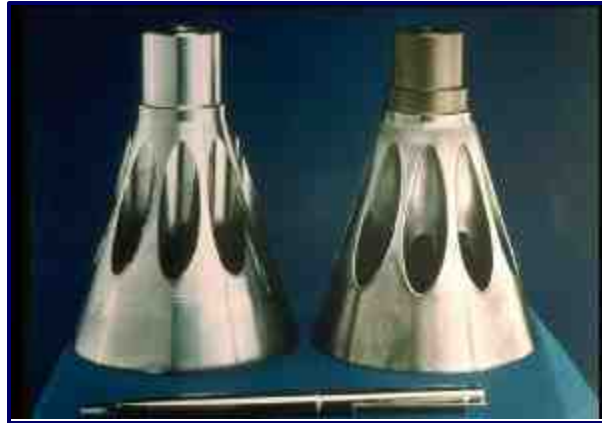
Figure 12 Cone With Electrolytic Formed Edges
