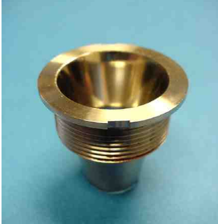
Figure 14 Internal surface polishing by Electrolytic Material Removal
