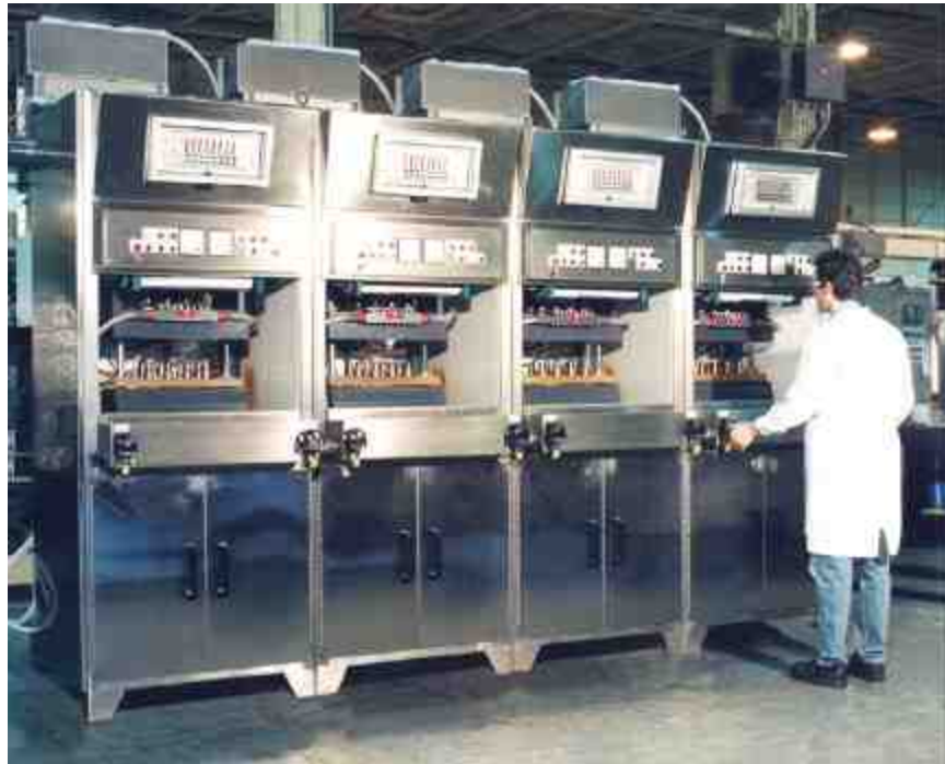
Figure 5 Four Station Modular Electrolytic Deburring System
