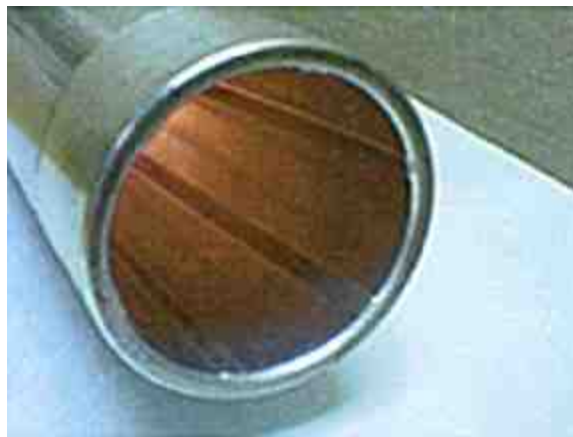
Figure 16 a Electrolytically Formed Rifling
