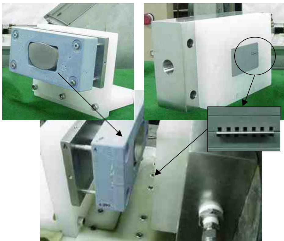
Figure 2: (upper left) photograph of workpiece, (upper right) stainless steel tool, (bottom) assembled fixture
