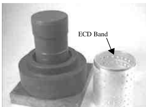
Figure 7. ID deburred with 6 electrodes.
