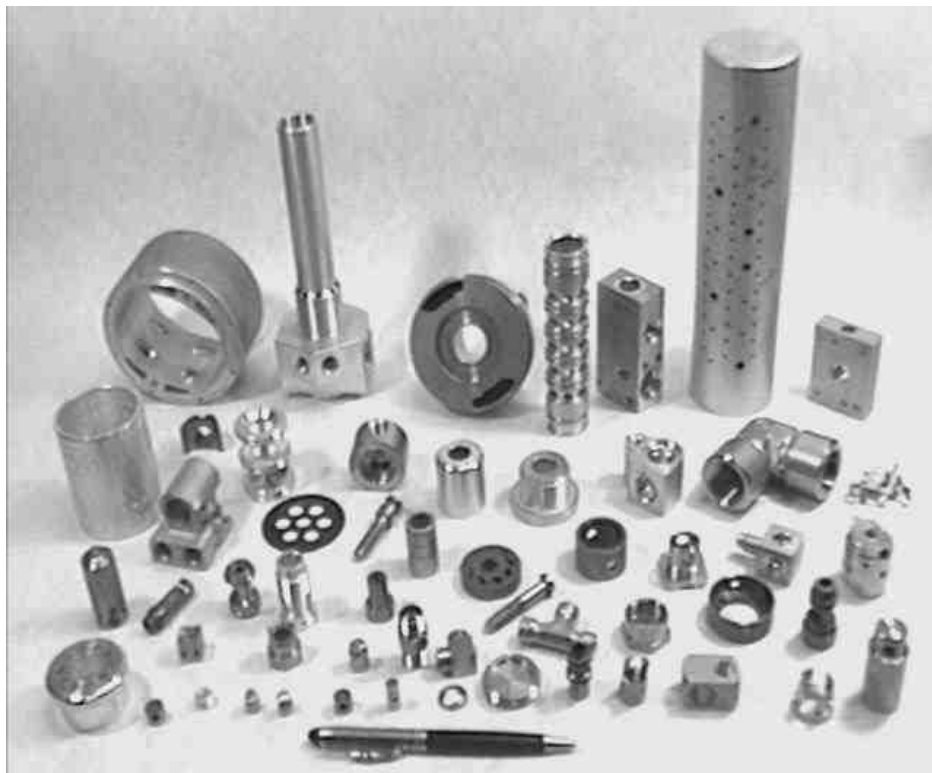
Figure 1. Assorted workpieces deburred using ECD.
