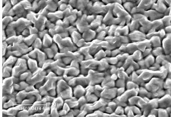
Figure 7: SEM image of electrodeposit surface after a potentiodynamic scan from OCP to  $-600$  mV SCE.
