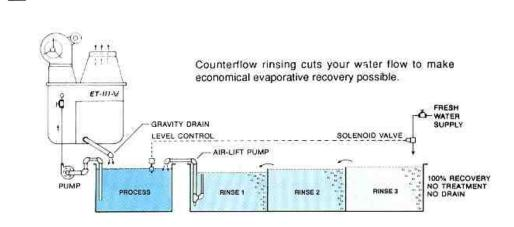
In this case, process solutions is circulated through an atmospheric evaporator at about 45 GPM and sprayed into an evaporation chamber where air is introduced, and then the solution returns via gravity back to the process tank. As the air passes through the evaporator, it is wormed from the contact with the worm solution. As it is wormed in direct contact with the solution it will pick up humidity.<sup>6</sup>
