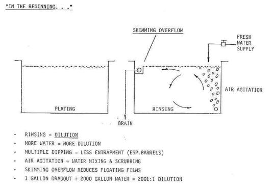
Water usage was not a concern. Drag-out was not a concern. As long as the parts were plated and cleaned all was well. In the illustration above, if the parts need to be cleaner, just turn up the faucet, and let the water over-flow down the drain, and later to waste treatment.
