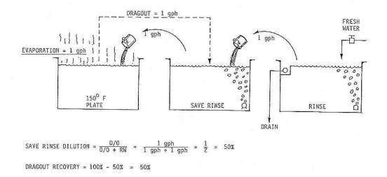
It is intuitive to reason that if the dragout of 1 GPH is mixed with 1 GPH of fresh water, then the mixture in the "save rinses" is at a 50% concentration level of the process tank.<sup>4</sup>
