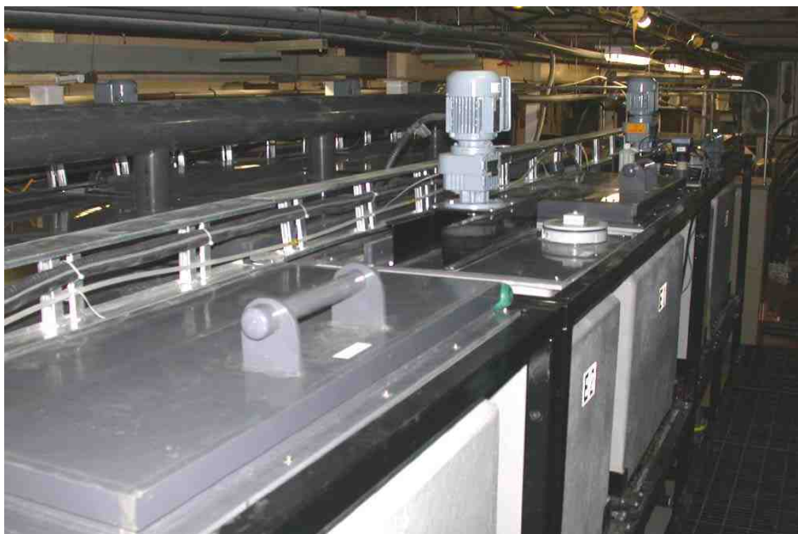
Figure 4. Mixer/Settler in A-LIX™ Prototype Plant
