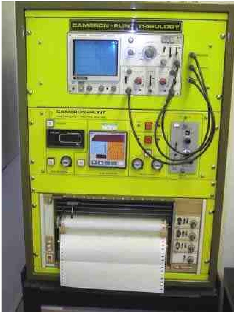
Control Panel with oscilloscope, power controls and chart recorder.
