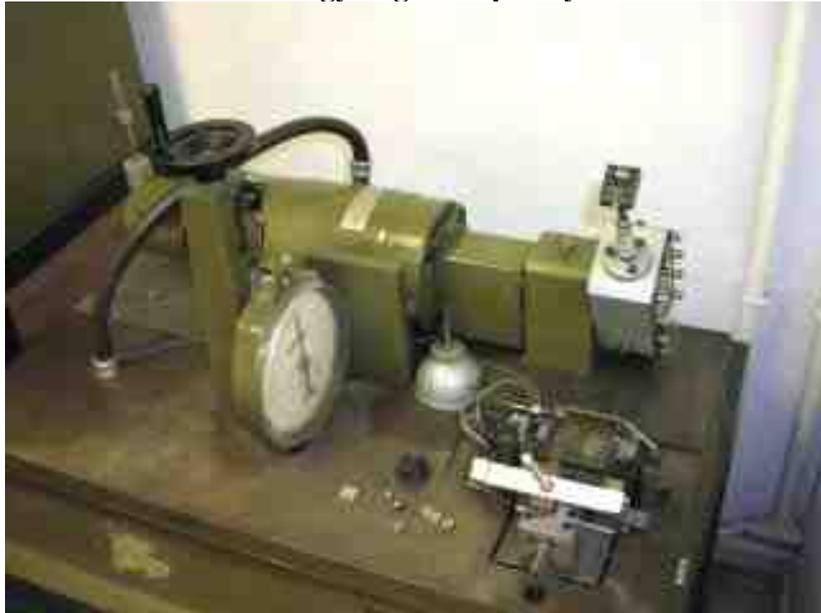
View showing motor, load gauge and open sample cell.
