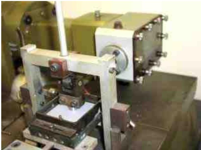
View showing sample cell with test plate and cylinder.
