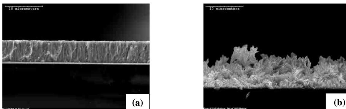
Figure 2 SEM SE images showing Au-Sn deposits obtained from an as prepared solution (a) and a solution that has been aged for 5 days (b). In both cases, pulse plating (2ms ON and 8ms OFF) at  $2.4 \text{ mA/cm}^2$  ( $2.23 \text{ A/ft}^2$ ) was used.
