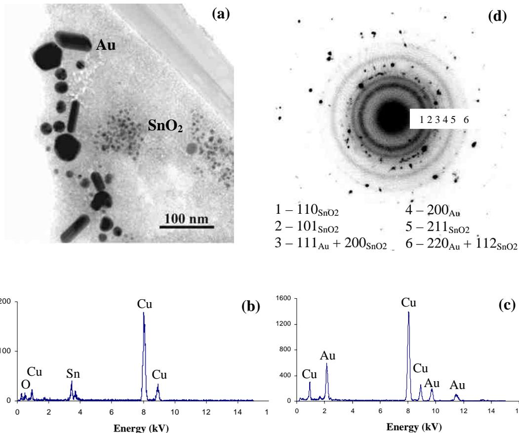
Figure 8 a) TEM BF image from a sample obtained from a suspension that developed on mixing individual Au and Sn solutions. b) EDX spectrum obtained from several of the smaller particles in (a). c) EDX spectrum from one of the larger particles in (a). d) SAD pattern from the region shown in (a). The continuous rings correspond to SnO<sub>2</sub> and the discontinuous rings to Au.
