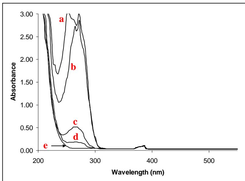
Figure 7 UV/Vis spectra obtained from a Au-Sn electroplating solution after ageing for: a) 0 hrs, b) 4.5 hrs, c) 22 hrs, d) 28 hrs and e) 46 hrs.
