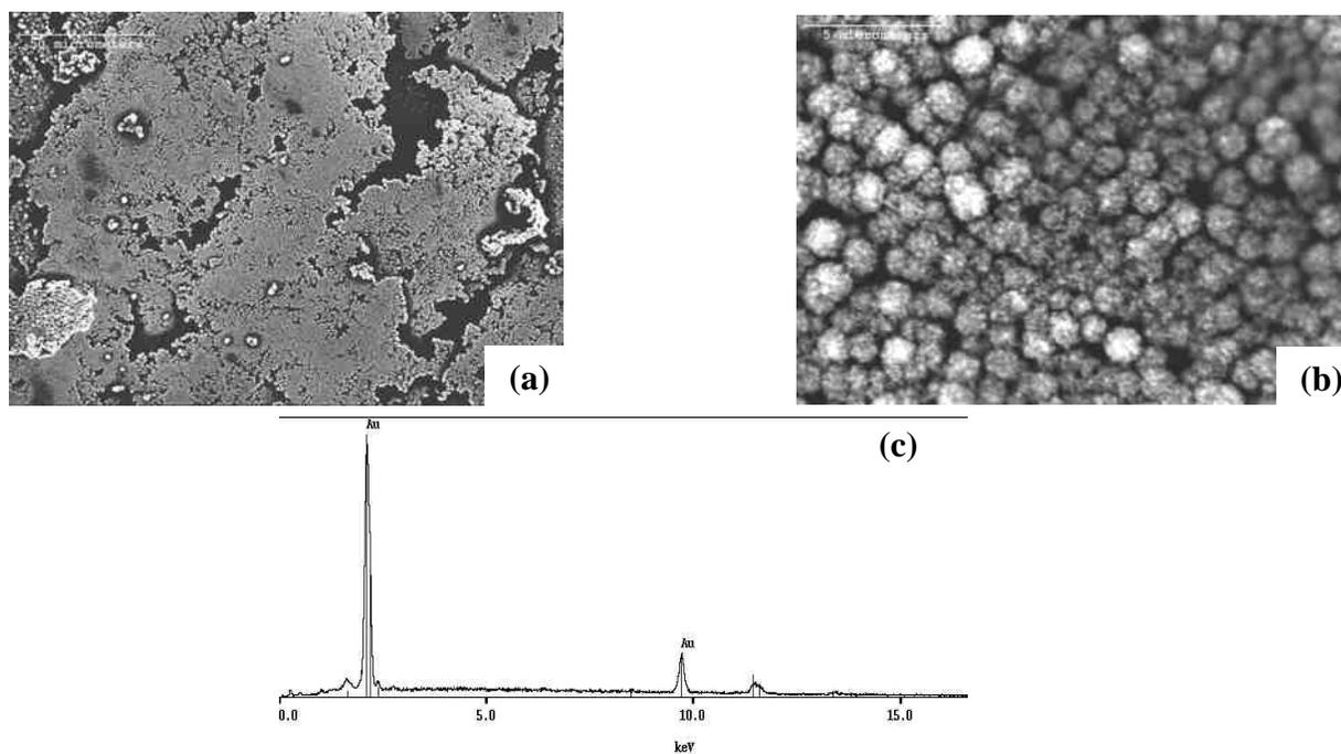
Figure 3 a) and b) SEM SE images of a precipitated film from a solution aged for 21 days. c) EDX spectrum from the region shown in (b).
