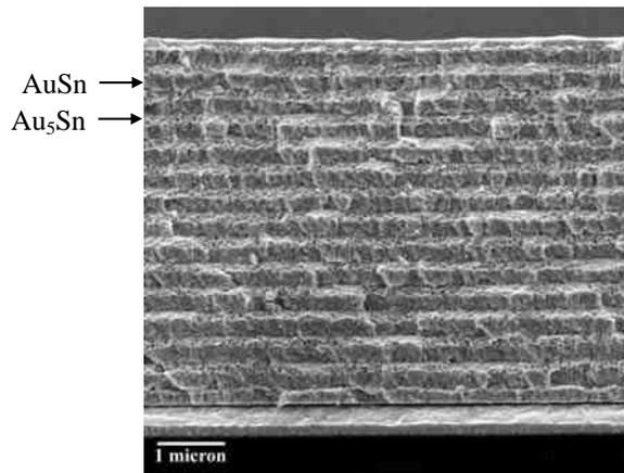
Figure 1 SEM secondary electron (SE) image showing an Au-Sn deposit with an overall composition of 30 at% Sn. The structure consists of alternating layers of  $\text{Au}_5\text{Sn}$  and AuSn, which were obtained by using alternate current pulses of  $0.8 \text{ mA/cm}^2$  ( $0.74 \text{ A/ft}^2$ ) and  $2.4 \text{ mA/cm}^2$  ( $2.23 \text{ A/ft}^2$ ) respectively.
