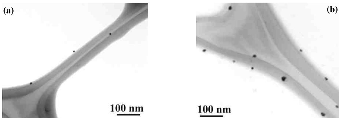
Figure 6 a) TEM BF image from a sample obtained from an as prepared Au-Sn solution. b) TEM BF image from a sample obtained from a Au-Sn solution aged for 2 days.
