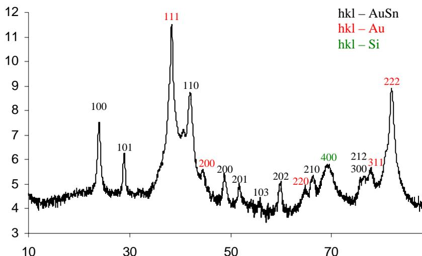
Figure 9 XRD spectrum from a Au-Sn deposit obtained from a plating solution aged for five days. The relative intensity is plotted on a log scale to accentuate the less intense peaks. The diffraction peaks can be indexed to AuSn and Au.
