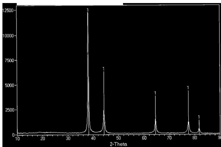
Figure 4 XRD spectrum from the precipitated film shown in Figure 3. All diffraction peaks can be indexed to metallic Au.
