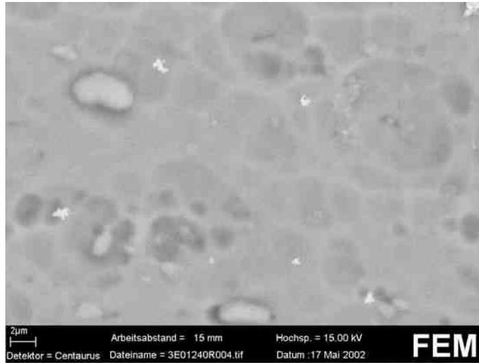
**FIGURE 6:** SEM-picture of an anodised aluminium surface (before immersion in the electrolyte)
