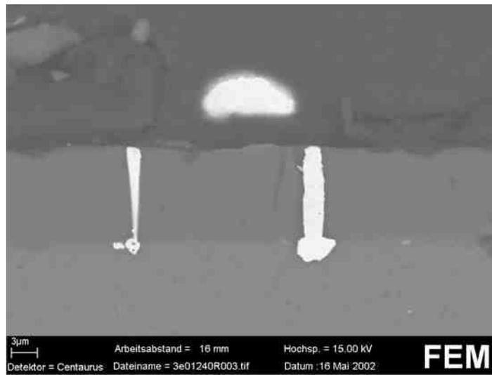
**FIGURE 9: SEM-picture of a cross-section of an anodised aluminium surface (after several hours electrodeposition)**
