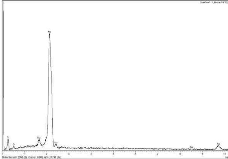
**FIGURE 23: EDS-spectrum of sample obtained from electrolyte 3; electrodeposition container: flow cell**
