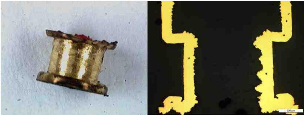
**FIGURE 15:** Myringotomy tube obtained from electrolyte 1; electrodeposition container: beaker
