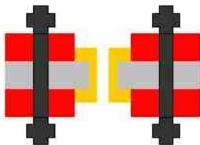
5) Disassembly, dissolution of aluminium in sodiumhydroxide, plastic sheets are reusable
