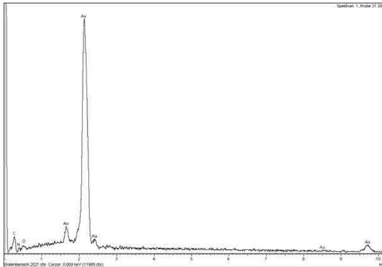
**FIGURE 22:** EDS-spectrum of sample obtained from electrolyte 2; electrodeposition container: flow cell
