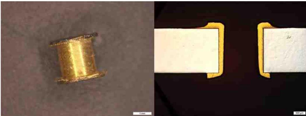
*FIGURE 18: Myringotomy tube obtained from electrolyte 2; electrodeposition container: flow cell*
