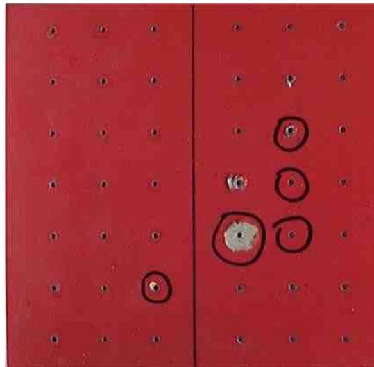
**FIGURE 11:** Lacquered AlMg1-sheet after laser drilling
