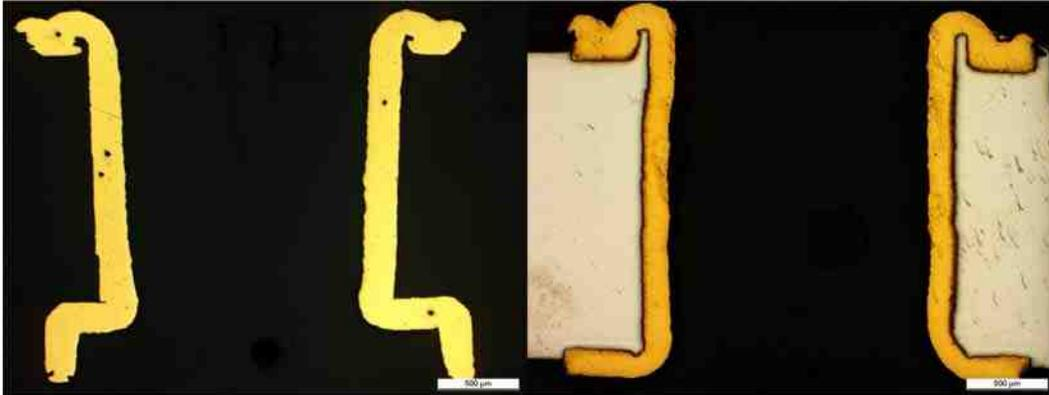
*FIGURE 17: Myringotomy tube obtained from electrolyte 2; electrodeposition container: beaker*
