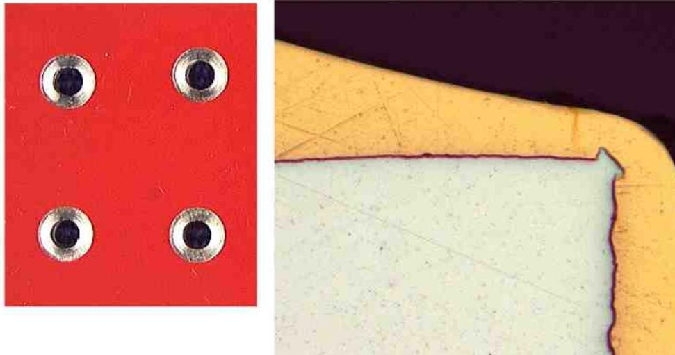
**FIGURE 12:** *Left: Top view of lacquered aluminium sheet, after mechanical precision drilling; right: cross-section of template corner*
