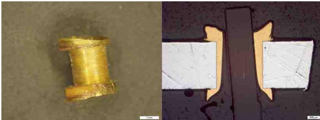
FIGURE 20: Myringotomy tube obtained from electrolyte 3; electrodeposition container: flow cell
