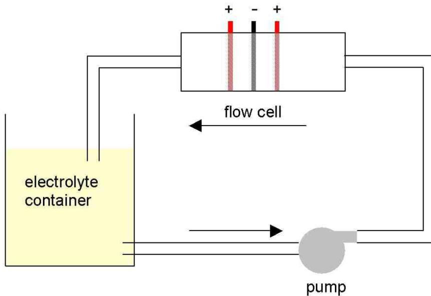
**FIGURE 14:** Flow cell (illustrated in a diagram)
