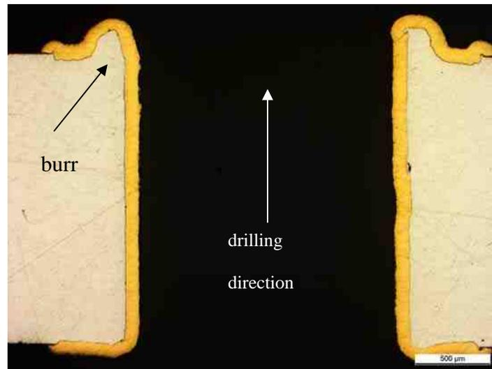
**FIGURE 10:** Cross-section of sample (template processing: mechanical drilling)
