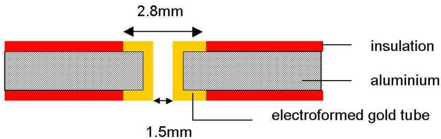
*FIGURE 3: Schematic cross-section of the electroformed gold tube*
