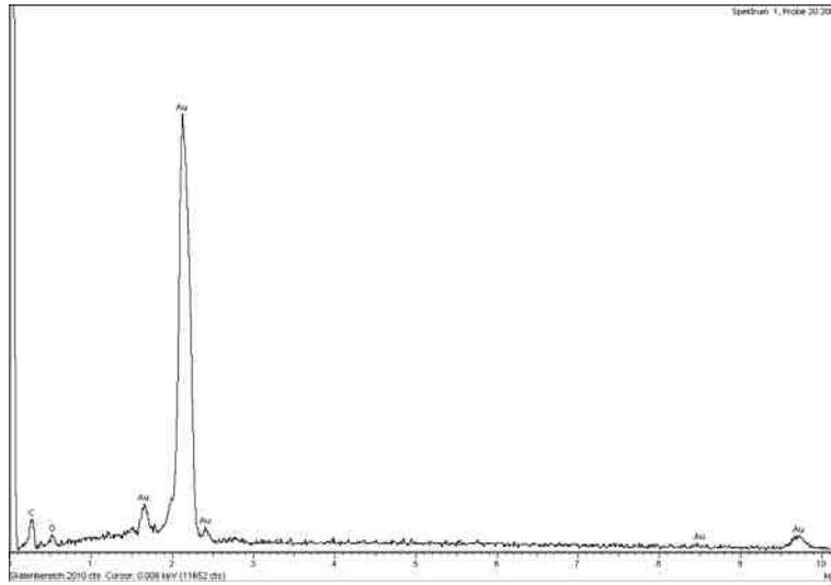
**FIGURE 21:** EDS-spectrum of sample obtained from electrolyte 1; electrodeposition container: flow cell
