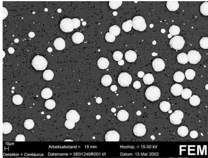
**FIGURE 8: SEM-picture of an anodised aluminium surface (after several hours electrodeposition)**
