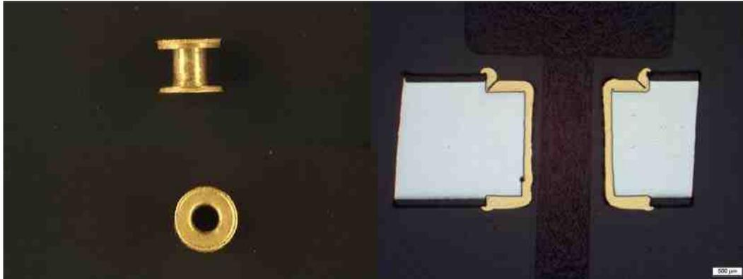
FIGURE 19: Myringotomy tube obtained from electrolyte 3; electrodeposition container: beaker
