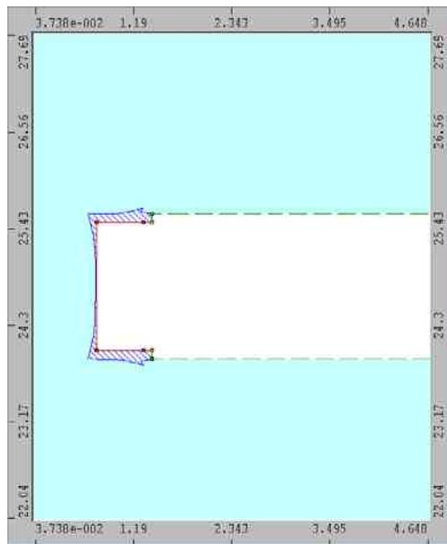
**FIGURE 4:** Current density map. The cross-hatched regions are proportional to the current density. The green regions represent insulated parts.
