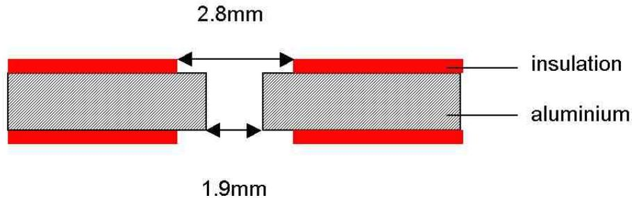
*FIGURE 2: Schematic cross-section of the aluminium template*
