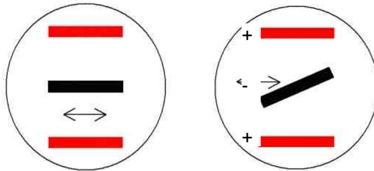
**FIGURE 13:** Top view of electrodes position in the electrolyte container (beaker); left: parallel, right: inclined (red: anodes, black: cathodes)
