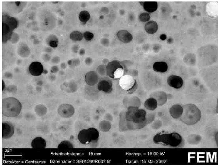
**FIGURE 7:** SEM-picture of an anodised aluminium surface (after several hours immersion in the electrolyte; no current)
