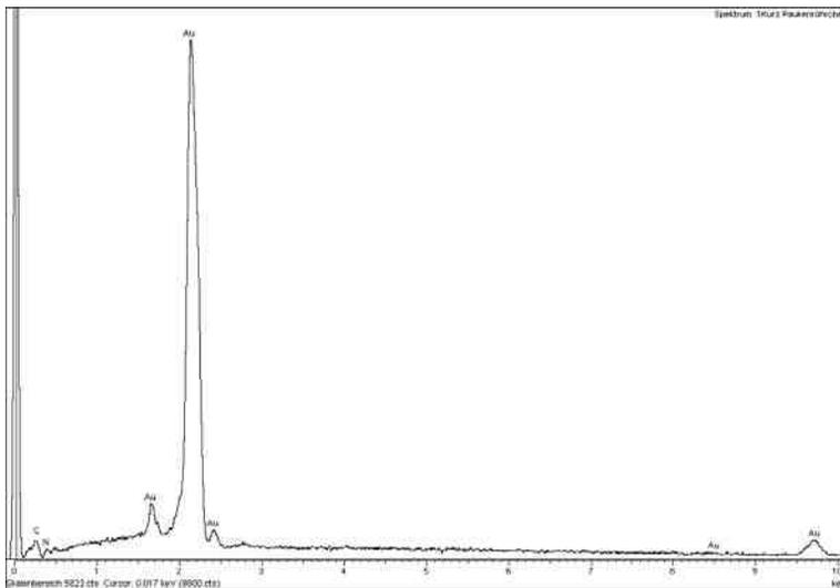
**FIGURE 24: EDS-spectrum of reference sample (gilded silver)**
