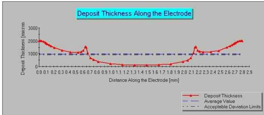
**FIGURE 5: Deposit thickness along the cathode**
