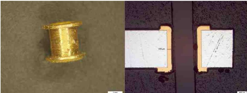
**FIGURE 16:** Myringotomy tube obtained from electrolyte 1; electrodeposition container: flow cell
