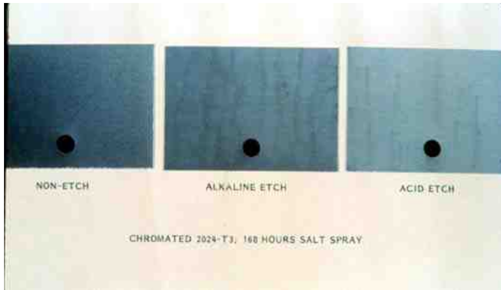
Figure 2 After 168 hours 5% salt spray. The non-etched (left) panel shows no corrosion. Others failed
