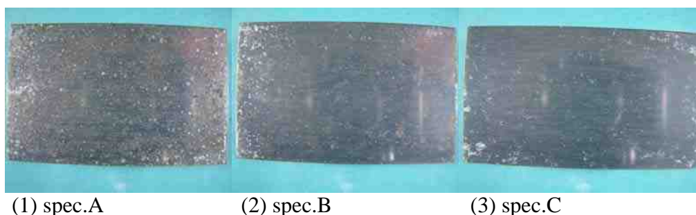
Fig.1 Surface conditions of Al-Cu alloys after CASS tests.
