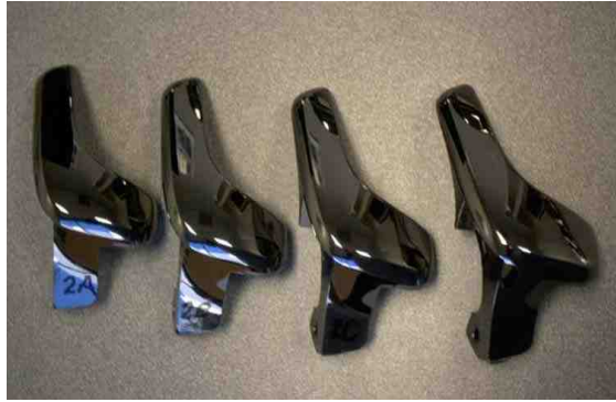
Figure 7 – Black tin-nickel plated PA door handles
