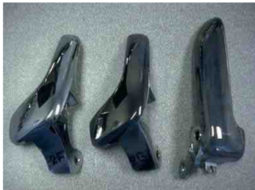
Figure 6 - PA door handles plated with black trivalent chromium
