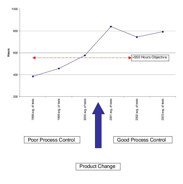
Resistance To Salt Fog Exposure (Adhesion)
