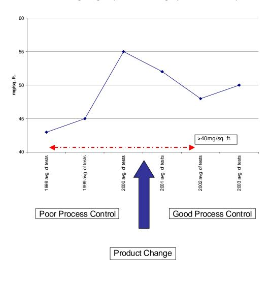
Coating Weights (measured in mg/square foot surface)
