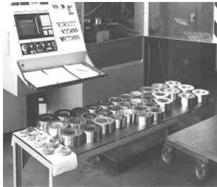
FIGURE 13 ECP POLISHED FLOW VALVES
