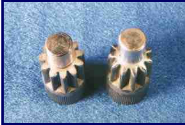
FIGURE 7 DEBURRING AND RADIUSING OF GEARS
