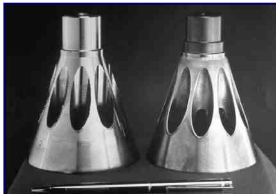
FIGURE 10 CONE WITH ELECTROLYTIC FORMED EDGES
