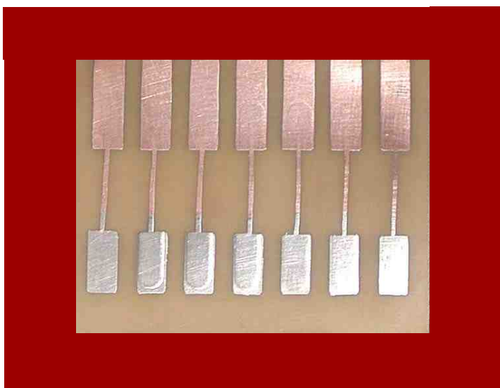
Fig. 5: The L-Cell plating template. Nickel plating on the pads is noted. The two pads at the edges serve as reference electrodes. The copper stripes feed the current to the pads. The larger copper pads on top serve as contacts.
