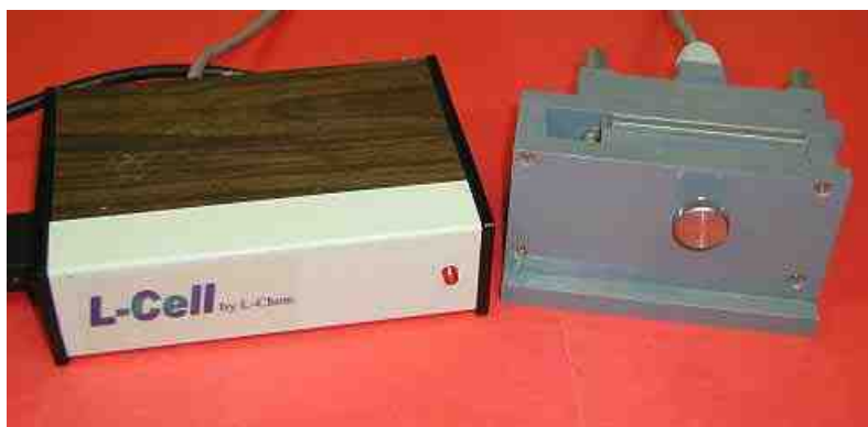
Fig. 7: The electronic control box (left) and the plating fixture (right) of the L-Cell
