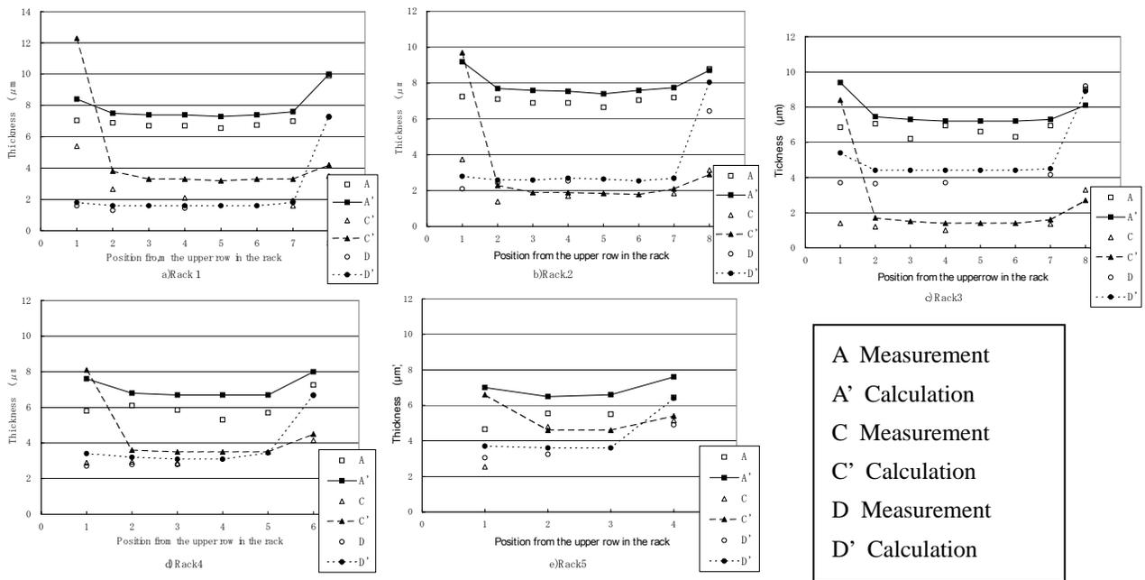
Fig. 8. Thickness comparison of racks
