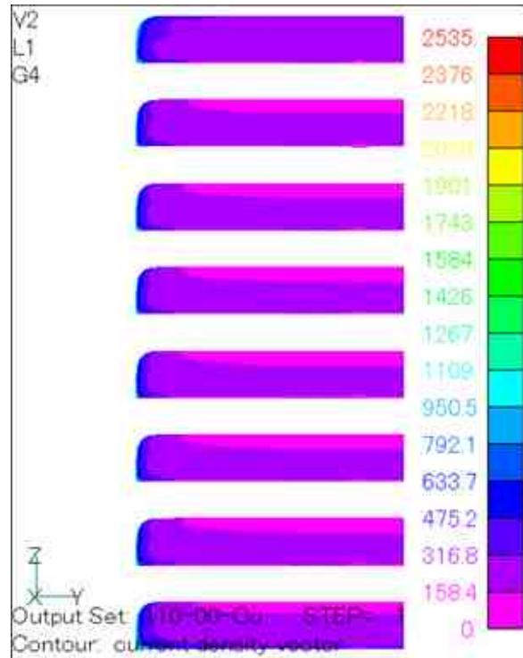
Fig. 5. Contour plot of current distribution on cathode ( $A/m^2$ )
