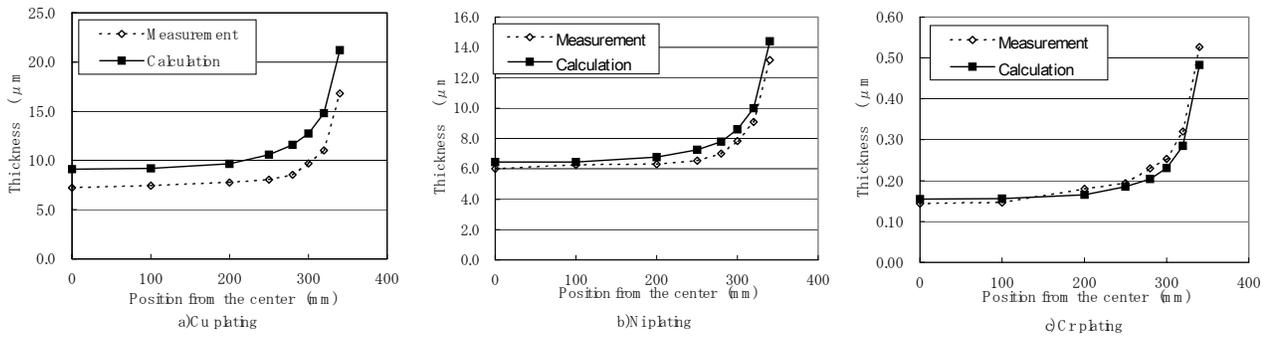
Fig. 7. Thickness comparison of the transverse direction
