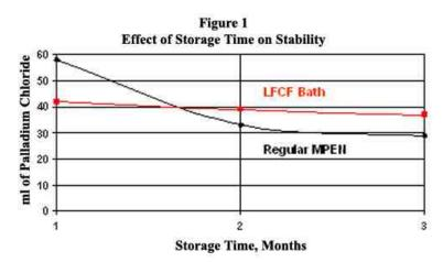
One supplier reported the stability of their solution as a function of the time that it was stored in a drum. Their intent was to determine whether the new lead-free stabilizer package degraded or lost effectiveness over time. The results of these tests are shown in Figure 1.<sup>19</sup> While initially, the lead free solution was less stable than the conventional bath, it maintained its stability better over time.
