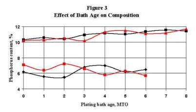
The phosphorus content of many electroless nickel coatings increase as their baths age. The coatings from LFCF baths behave the same way. Figure 3 shows the effect of bath age on the
