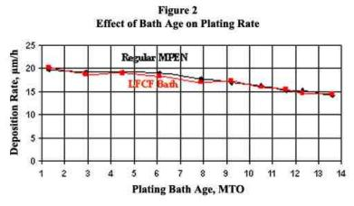
**Plating Rate.** An adequate plating rate is a critical characteristic of a bath. It determines the applicator's productivity. If the rate of a bath is low, the applicator will be reluctant to use it. Fortunately, the deposition rate of the LFCF baths is very similar to that of conventional
