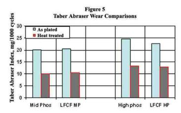
The hardness and wear resistance of LFCF and conventional coatings should be similar since the coatings' basic structure is unchanged. It is the relative amounts of crystalline and amorphous phases present that determines hardness and wear resistance.<sup>24</sup> These phases and structure are a function of the coating's phosphorus content. Additives like lead and cadmium have little effect on structure.
