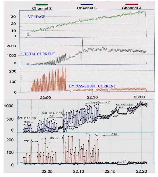
Check the net gain of 195Amps at 22:07, which is a 115% increase above 170 Amps without CSD. Another net increase of 270 Amps or 45 % above 600 Amps is recorded at 22:13 (end of pulse ramp.)
