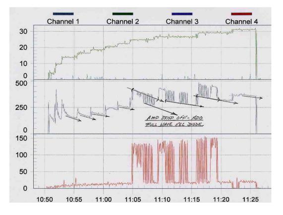
The amperage drop off (ADO) rate is increased to such a considerable degree that it is enough to be a significant improvement for the process cycle. Anodize operators know that faster amperage decay can be beneficial when running 2000 series alloys like 2024.
