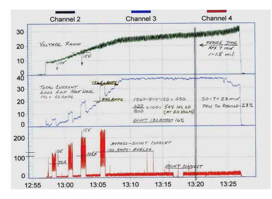
Please check the net gain of 430 amps at 13:06 with a 54% increased current density using CSD. This same process cycle can be used on 2024 and 7075 passing Taber Abrasion requirements per MIL-A-8625 F.
