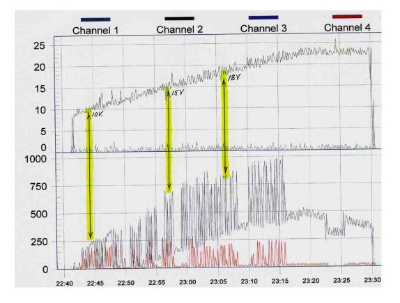
The Amperage gain is well over 50% in this extreme case as you can see from the turn off or interruption periods. There is always a small CSD unit that is operational during the entire anodize cycle with no pulse applied. You can note the amperage drop when this section is disconnected at 23:23 for 3 minutes. Please note – CSD specifications will also be included in this paper as they are integrated with the PSR technology.
