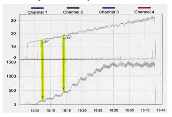
This example was taken from a production run of commercial parts requiring 2.0-2.5 mils hard anodize. The PSR was set for a step ramp with a one min dwell and one min ramp. Please note - all PSR operating specifications will be included in this paper.
