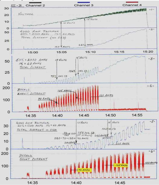
Please note the 75% and 106% increase in current density at 10 and 15 volts respectfully (data logger graphs 3 and 5).
