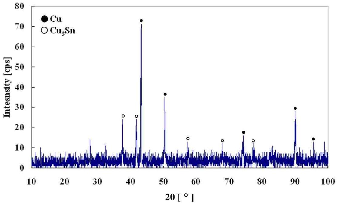
Fig.5 XRD for the specimen heat treated at  $250^\circ\text{C}$  ( $482^\circ\text{F}$ )
