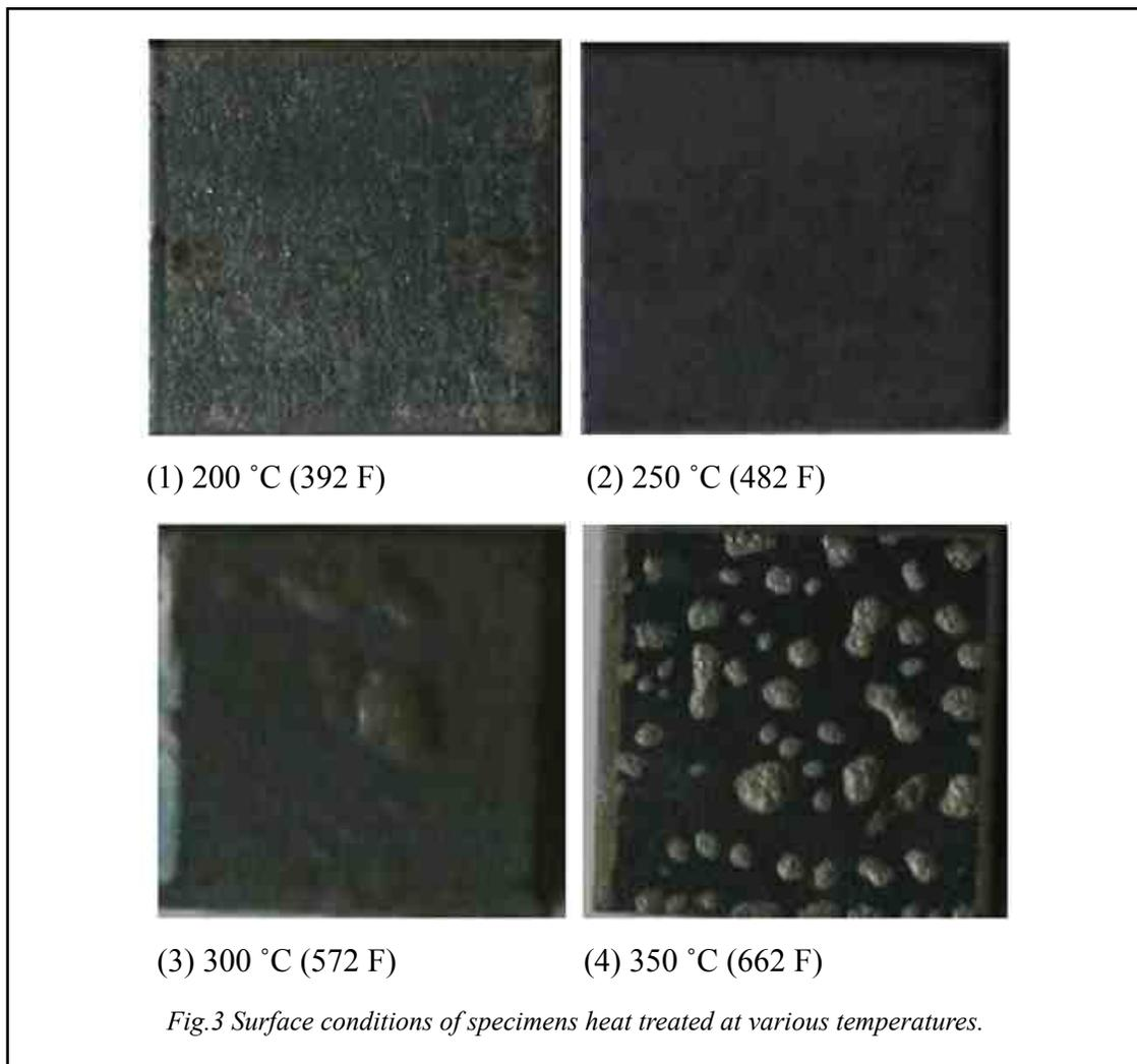
shapes. As for the change by heat treatment, we could observe that any change didn't occur at 200 degrees Celsius (392 degrees Fahrenheit, Fig.3-(1)) and that the nucleation became more obvious with increasing temperatures. Focusing on the correlation between the nucleation and thickness of the original surface stacked layers, we made clear that the tendency mentioned above became remarkable with increasing thickness.
