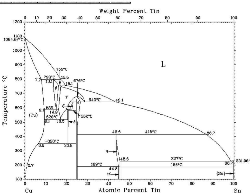
Fig.9 Phase diagram of tin and copper.
