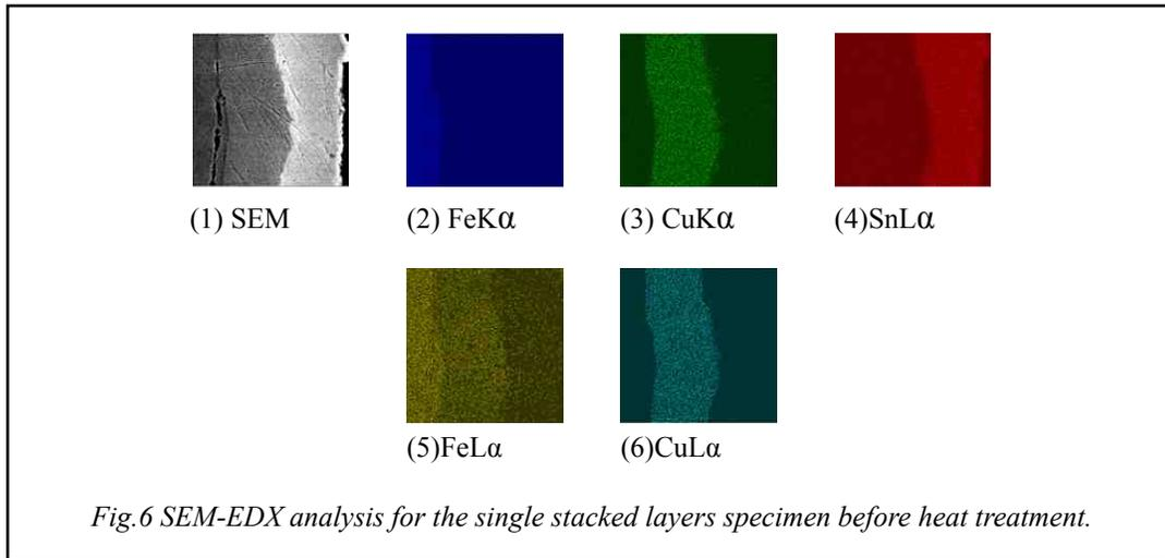
upper part of each figure, a SEM image, the element mappings for iron (K $\alpha$ ), copper (K $\alpha$ ), tin (L $\alpha$ ) are aligned from left to right, while the element mappings for
