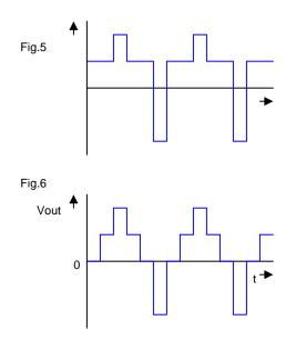
One aspect, using pulse waveforms, that is sometimes overlooked is cable induction. Cable induction has a negative effect on rise and fall times of pulse signals. The higher the induction of the cable, the less 'rectangular the output waveform of the rectifier will be.( see Fig. 7). To get the best possible waveforms you therefore want to use a low inductance cable like for example a coax cable.
