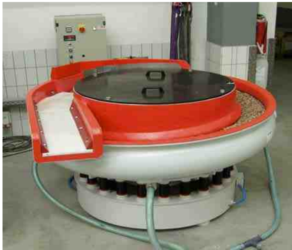
Image 4; Shows a traditional vibe bowl with parts/media separation deck. Ideal for processing short stubby parts such as gears, tappets and bearings.
