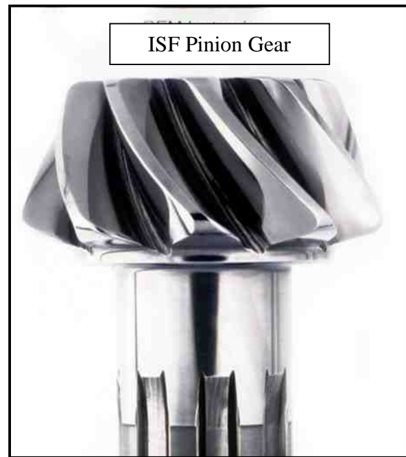
Image 12; Shows the same spiral differential pinion as shown in image 6. Note, grind line asperities have been removed leaving a smooth ISF.
