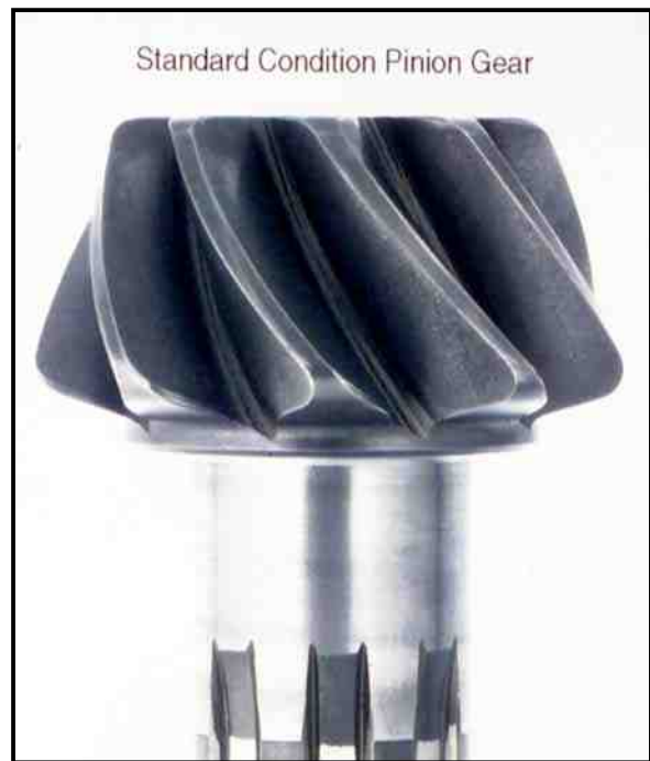
Image 6; Image of a differential pinion in traditional as ground finish. Note grind lines on the gear teeth.
