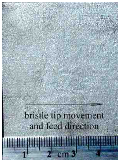
Figure 10 Post-treated surface generated by bristle blasting of flat rolled steel (condition B, appearing in Figure 8)
