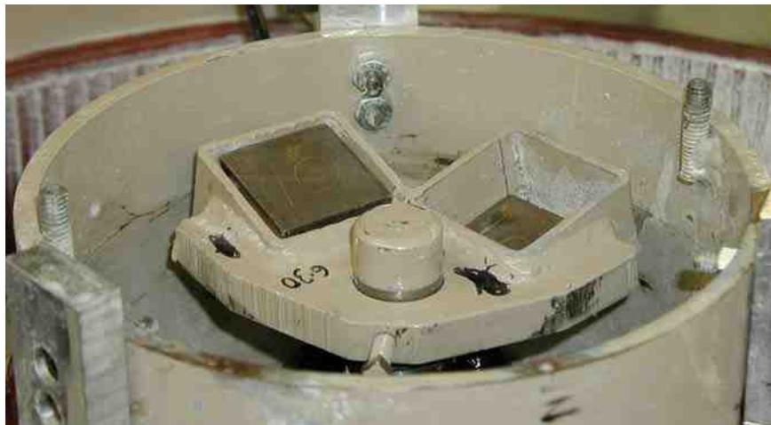
*Figure 3. Top weight cups used to control acceleration in the Rotofinish vibratory bowl.*
