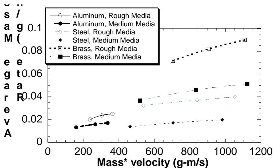
Figure 7. Comparison of mass-velocity on material removal rate.
