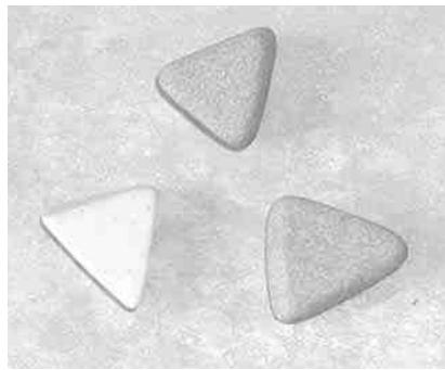
*Figure 4. Triangular ceramic media used in the investigation.*
