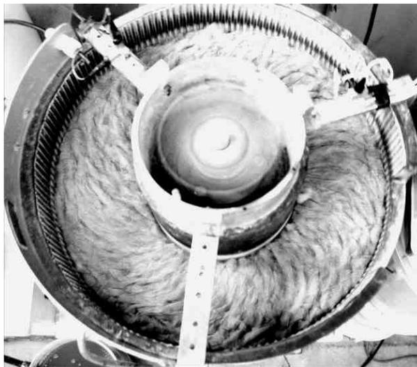
Figure 2. Representative flow pattern of the workload in a vibratory bowl.
