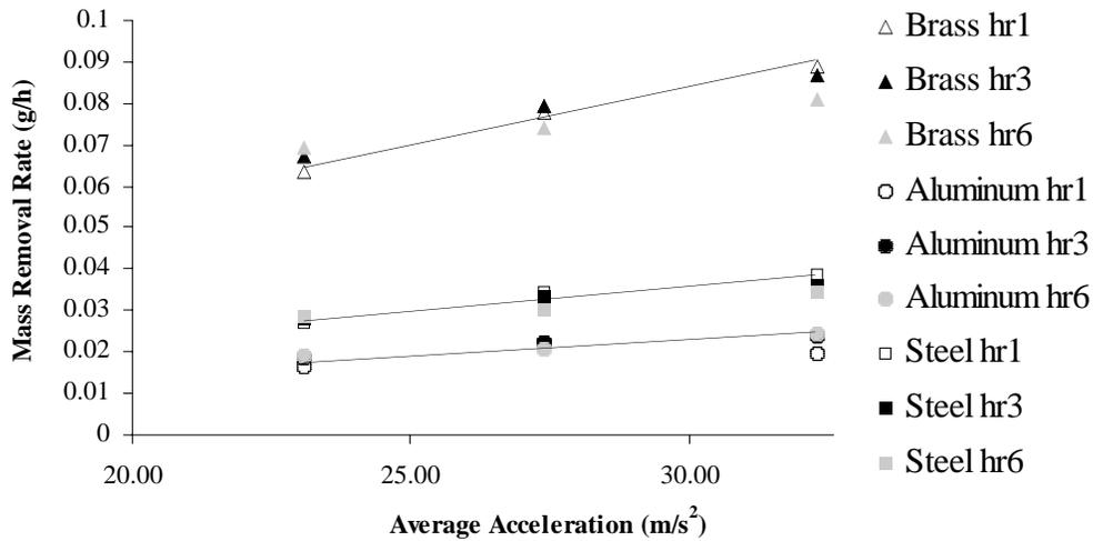
Figure 6. Material removal rates as a function of accelerations for brass, steel, and aluminum workpieces used in the study. Acceleration is expressed as multiples of the gravitational constant.
