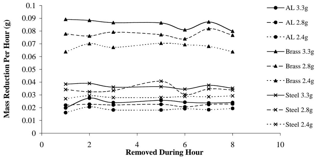
Figure 5. Material removal rates at various bowl accelerations over an 8 hour period for the fast cut media.
