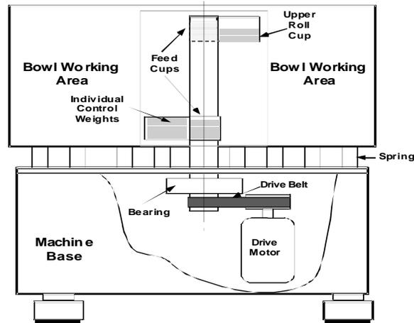
Figure 1. Schematic of a typical vibratory bowl machine.
