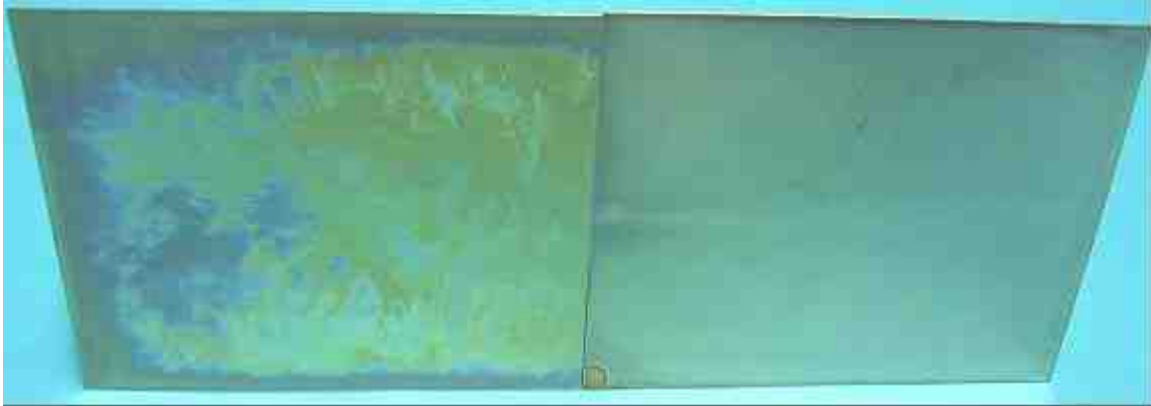
Fig. 7: Steel coupon (DC01 steel, 10 cm x 10 cm) after immersion into a Cr(III) passivation bath 6 . Left: Without addition of a corrosion inhibitor. Right: With 0.01% w/w cationic polyurea CP as bath additive.
