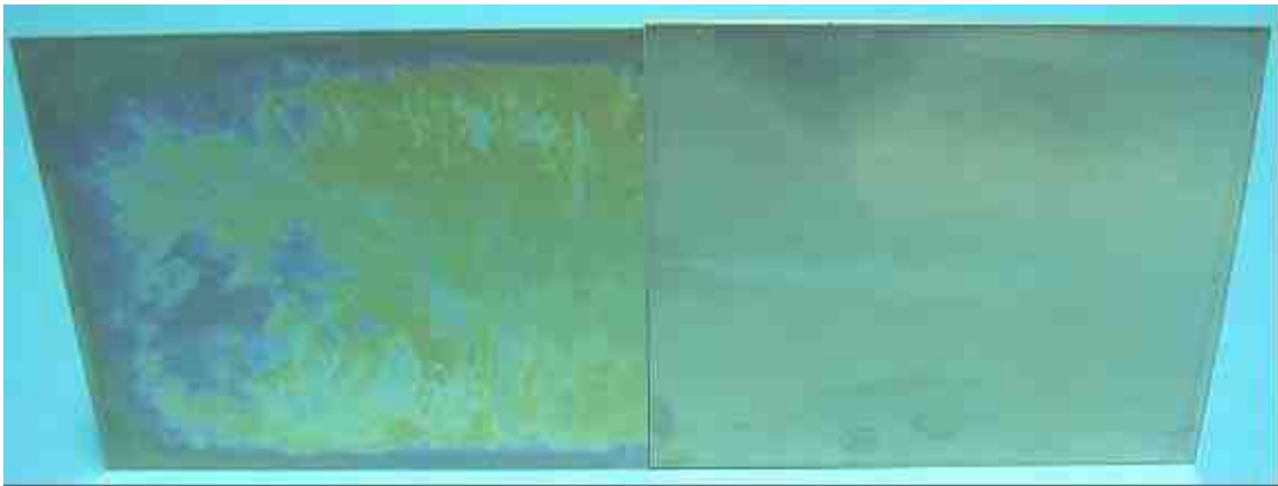
Fig. 8: Steel coupon (DC01 steel, 10 cm x 10 cm) after immersion into a Cr(III) passivation bath 6 . Left: Without addition of a corrosion inhibitor. Right: With 0.1% w/w cationic polyurea CP as bath additive.
