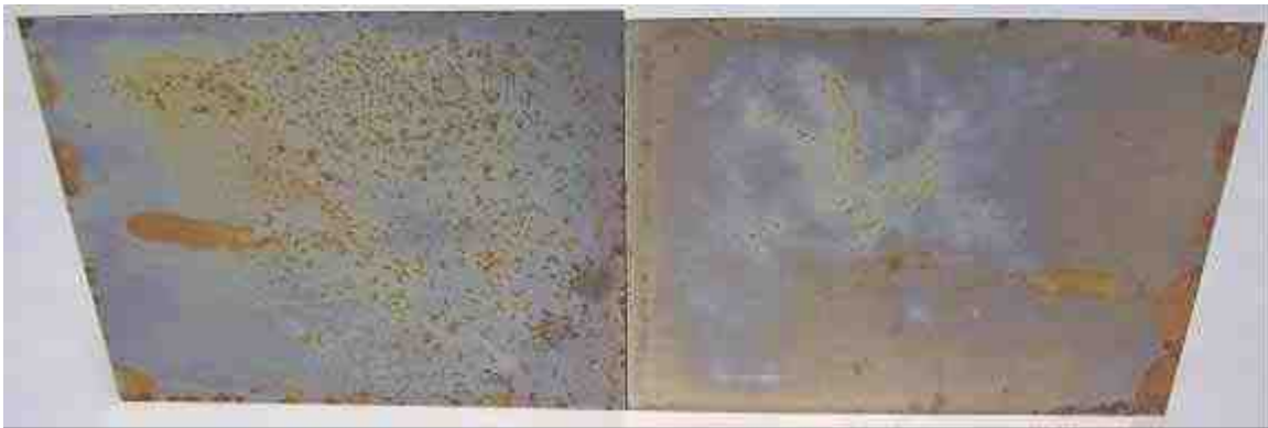
Fig. 12: Steel coupon (DC01 steel, 10 cm x 10 cm) after immersion into a Cr(III) passivation bath 6 and subsequent exposure to a humid-dry cycle. Left: Without addition of a corrosion inhibitor. Right: With 0.01% w/w ethinylcarbinol propoxylate PP as bath additive.
