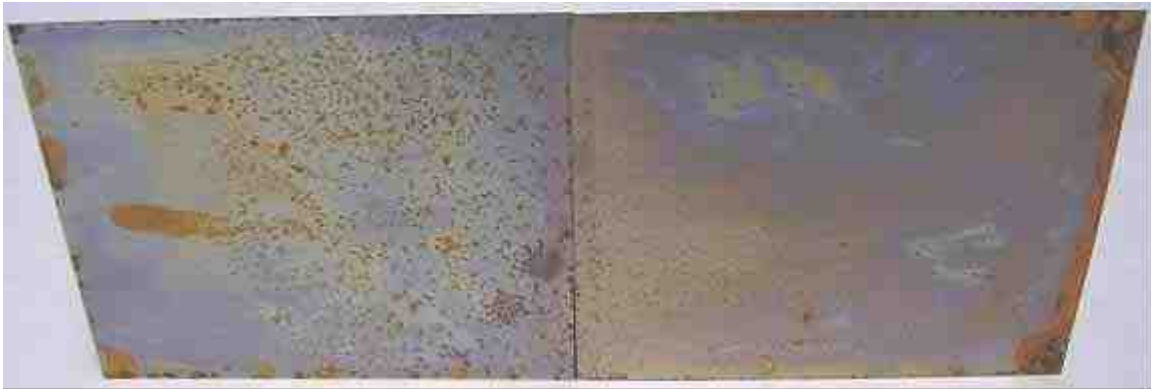
Fig. 10: Steel coupon (DC01 steel, 10 cm x 10 cm) after immersion into a Cr(III) passivation bath 6 and subsequent exposure to a humid-dry cycle. Left: Without addition of a corrosion inhibitor. Right: With 0.01% w/w cationic polyurea CP as bath additive.
