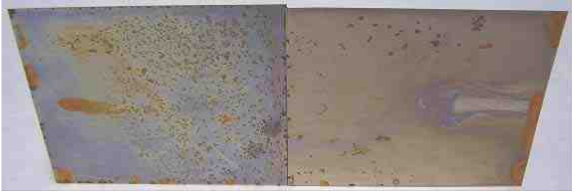
Fig. 13: Steel coupon (DC01 steel, 10 cm x 10 cm) after immersion into a Cr(III) passivation bath 6 and subsequent exposure to a humid-dry cycle. Left: Without addition of a corrosion inhibitor. Right: With 0.1% w/w ethinylcarbinol propoxylate PP as bath additive.
