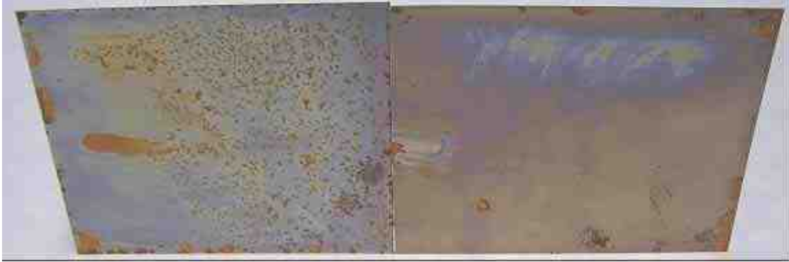
Fig. 11: Steel coupon (DC01 steel, 10 cm x 10 cm) after immersion into a Cr(III) passivation bath 6 and subsequent exposure to a humid-dry cycle. Left: Without addition of a corrosion inhibitor. Right: With 0.1% w/w cationic polyurea CP as bath additive.
