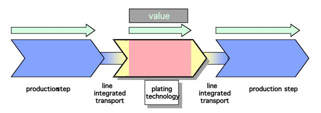
Hard chromium plating is a good choice for this type of process because only one chromium electrolyte is necessary. It is applicable for cleaning, pickling (electrolytic or electroless), predip/activation, and chromium plating. Due to the lack of transportation, no temporary corrosion protection is required as the production takes place in the same area.
